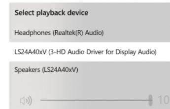
If only the HDMI or DP cable is connected from your monitor to the computer, only one speaker named **LS24A40xV** from the monitor will show in the Sound setting interface.
