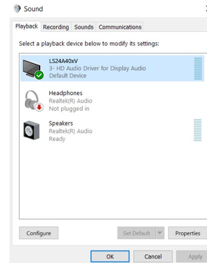
If the USB cable and the HDMI or DP cable are connected from monitor to the computer, two speakers named **LS24A40xV** and **Speakers (LS24A40xV)** respectively from the monitor will show in the **Sound** setting interface. The difference between **LS24A40xV** and **Speakers (LS24A40xV)** is only different signal source. You can choose either one to set as the default speaker for monitor.
