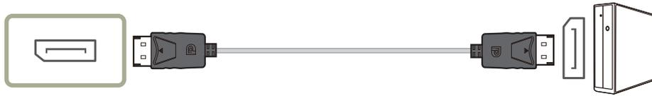
— A DP cable shorter than 1.5 m in length is recommended. Using a cable longer than 1.5 m can affect the picture quality.
