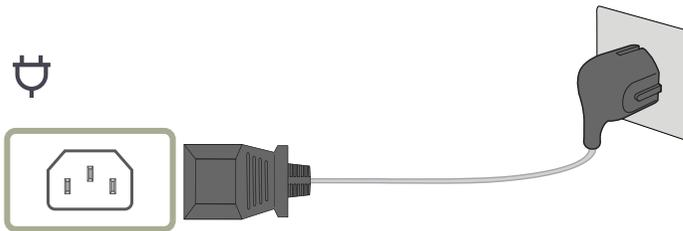
To use the product, connect the power cable to a power outlet and the
