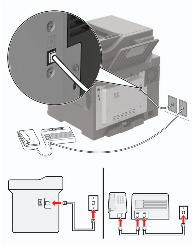
**1** Connect one end of the telephone cable to the line port of the printer.
