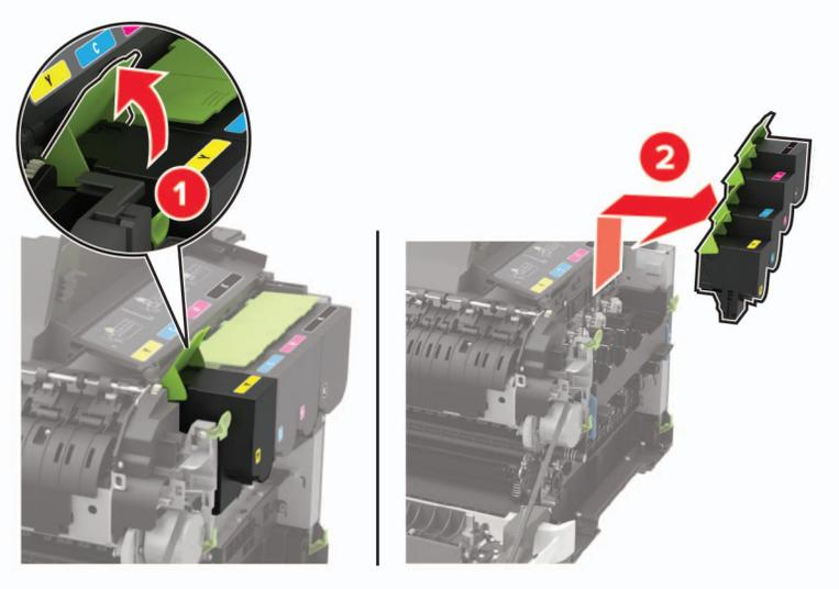
**6** Remove the used imaging kit.
