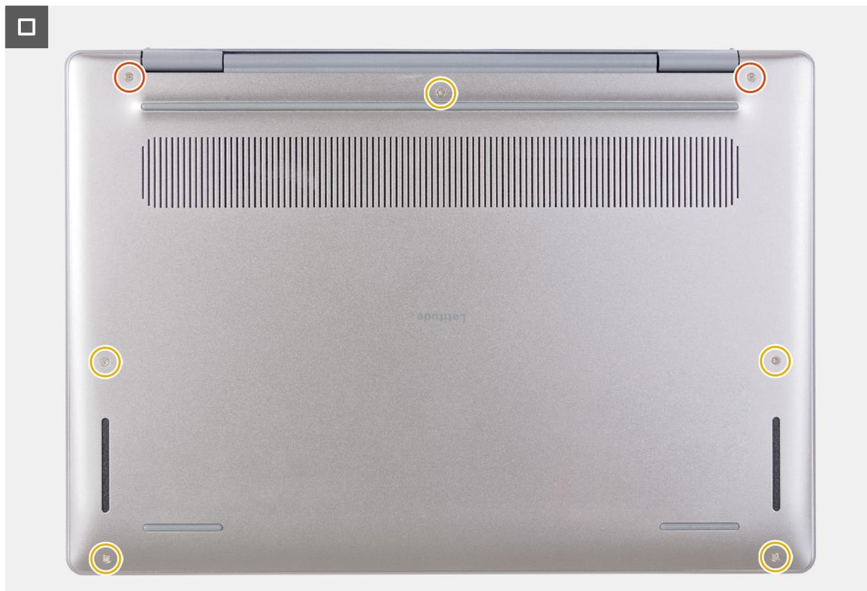
**Figure 15. Tightening and replacing the screws**
