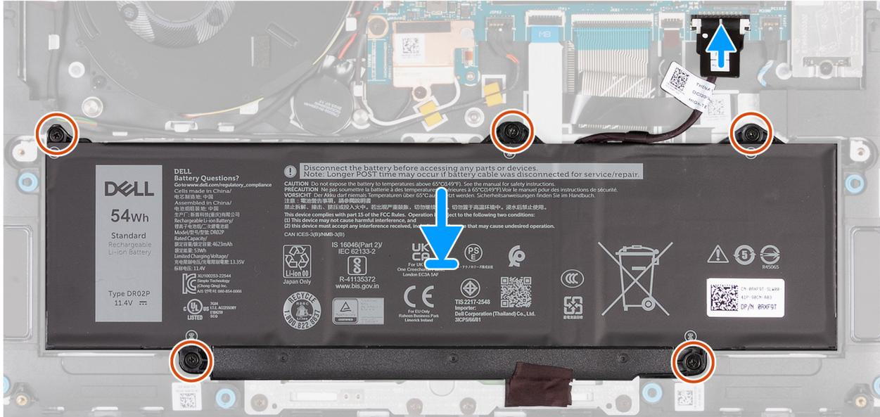
Figure 28. Installing the battery
