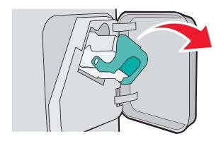
Use the metal tab to lift the staple guard, and then remove any loose staples.
