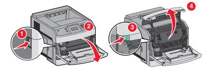
**3** Lift and pull the print cartridge out of the printer.
