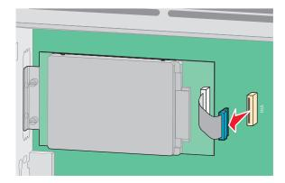
**b** Remove the screws holding the printer hard disk in place.
