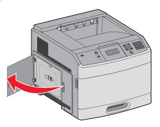
**2** Loosen the screw on the system board cover.
