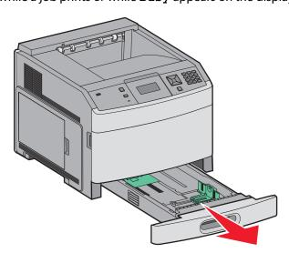
**2** Squeeze the width guide tab inward as shown, and move the width guide to the correct position for the paper size being loaded.
