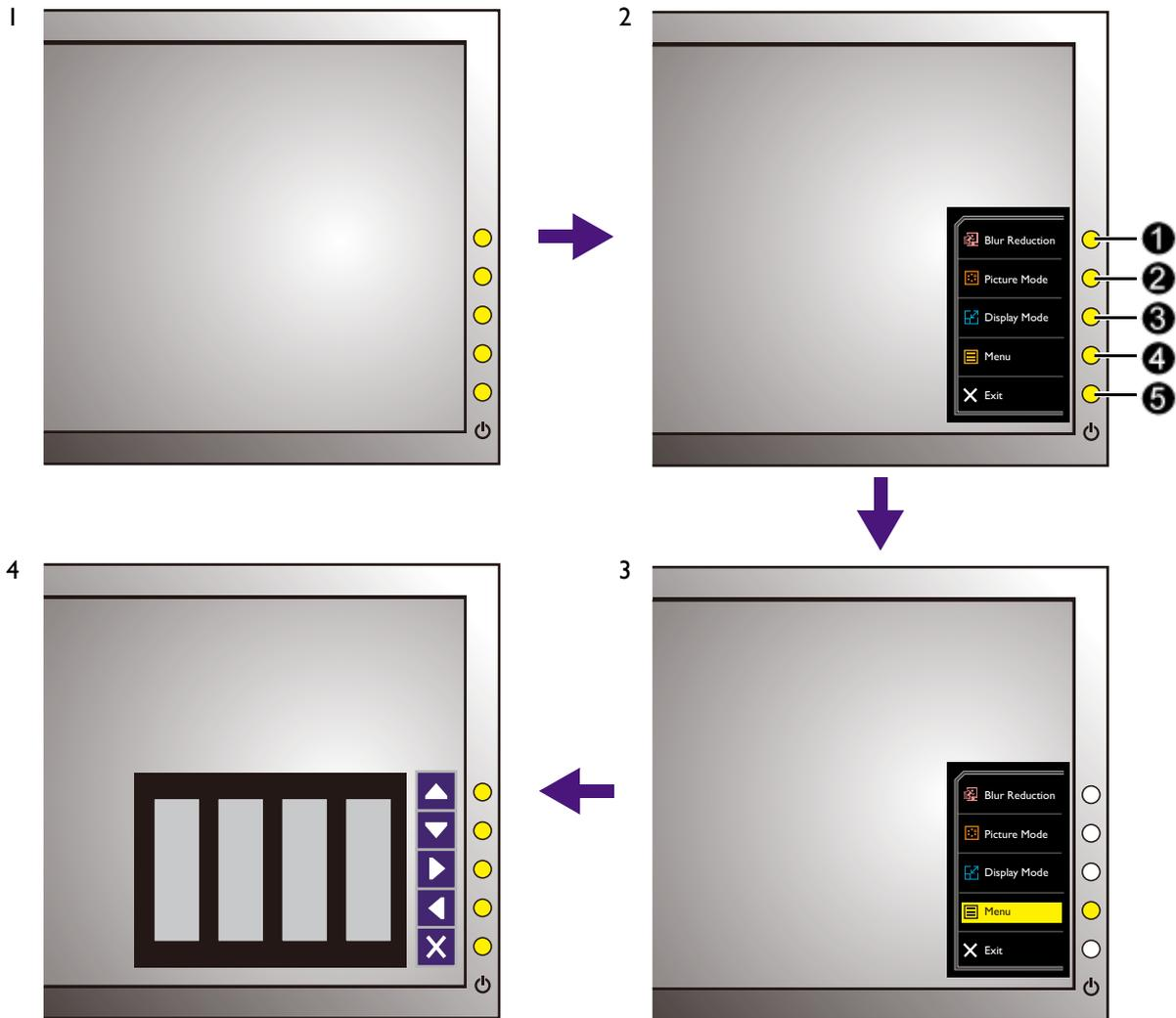
1. Press any of the control keys. Alternatively, press the wheel or the return button on the S Switch.
