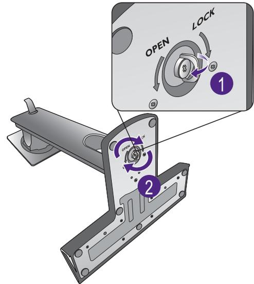
Orient and align the stand arm with the monitor (1), push them together until they click and lock into place (2).
