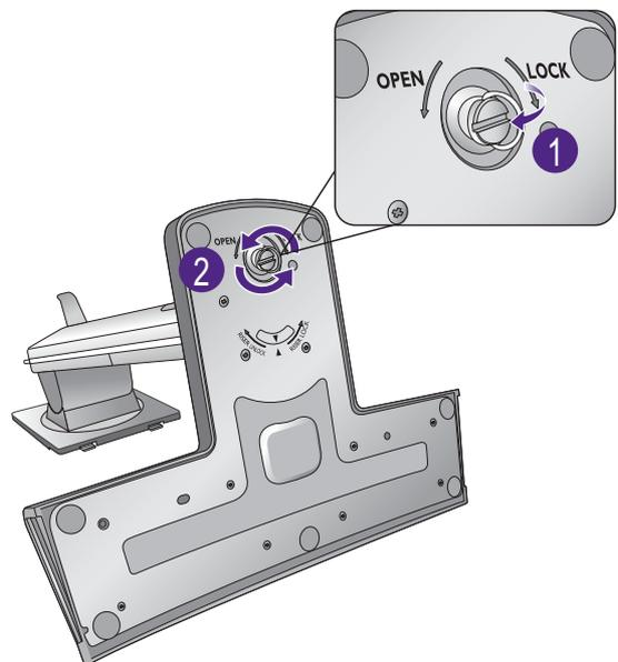
Turn the stand clockwise so that the arrow on the bottom of the stand points to **RISER UNLOCK** (1). And then detach the base from the stand (2).
