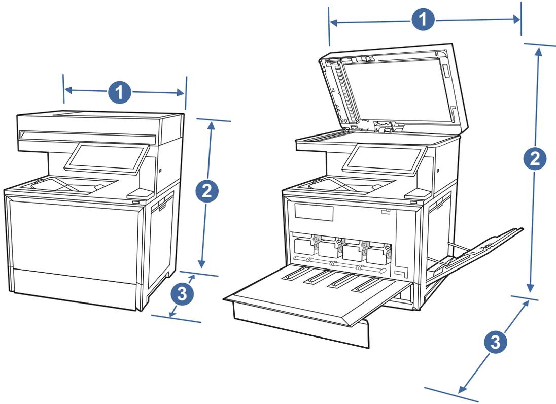
**Table 1-9 Dimensions for the printer (dn and zf models)**
