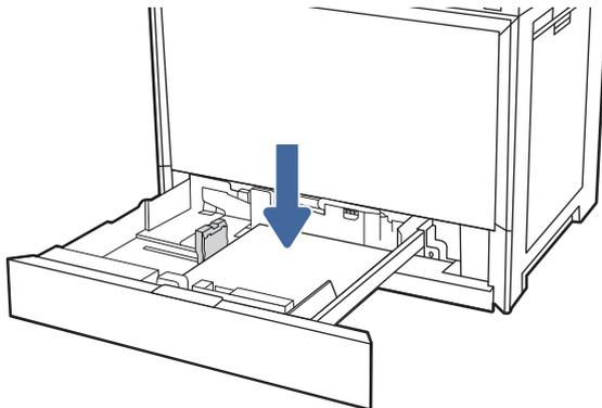
5. Adjust the paper-length and paper-width guides to the size of the paper being used. Check the paper to verify the guides lightly touch the stack, but do not bend it.
