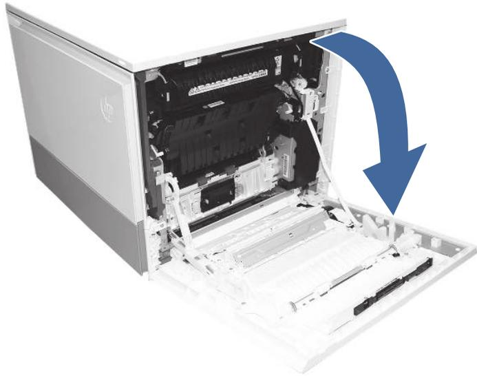
2. Remove the fuser and remove any jammed paper found.
