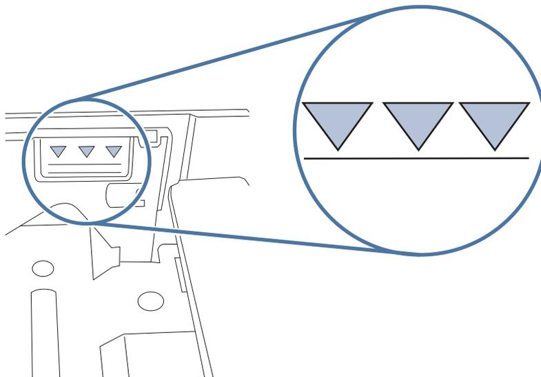
6. Make sure the paper guides in the tray are adjusted correctly for the size of paper. Adjust the guides to the appropriate indentation in the tray. The arrow on the tray guide should line up exactly with the marking on the tray.
