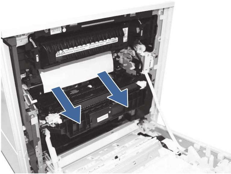
3. Remove the fuser and remove any jammed paper found.
