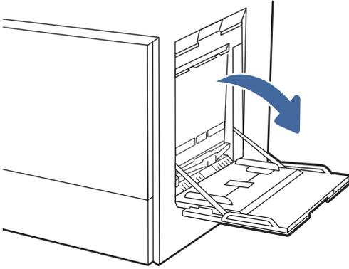
2. Pull out the tray extension to support the paper, if necessary.
