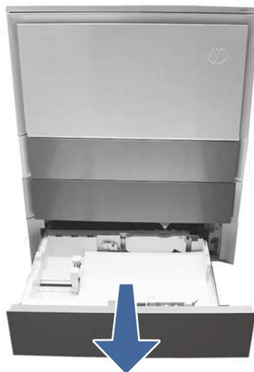
8. Remove the paper from the tray and discard any bent, curled, or damaged sheets.
