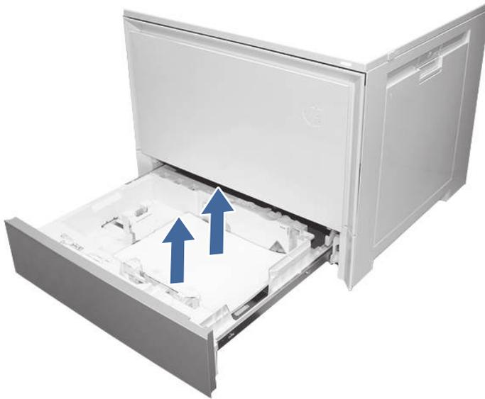
6. Make sure that the tray width and length guides are set to the correct paper size for the paper being installed into the tray and that the tray is not over filled above the fill mark (line below 3 triangles on rear guide).
