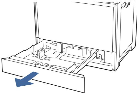
2. Before loading paper, adjust the paper-width guides by holding down the blue lock/unlock toggle switch on the rear paper-width guide, pinching the blue adjustment latch on the front paper-width guide, and then sliding the guides to the fully open position.
