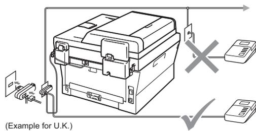
**Set the receive mode to External TAD if you have an external answering machine. See *Choose a Receive Mode* on page 6. For additional details, see *Connecting an external TAD* in the *Basic User's Guide*.**
