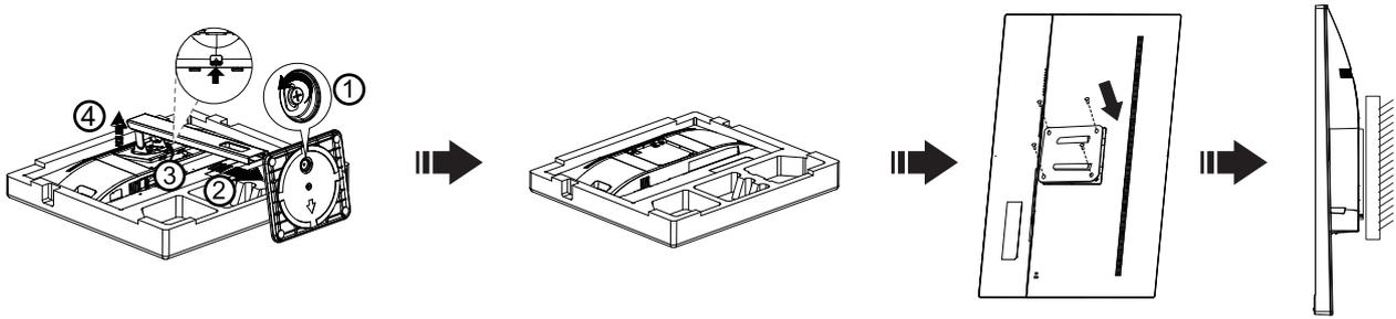
This monitor can be attached to a wall mounting arm you purchase separately. Disconnect power before this procedure.
