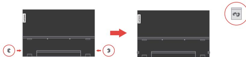
3. Attach the mounting bracket from the wall mounting kit to the monitor.
