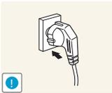
Insert the power plug all the way in so it is not loose.
