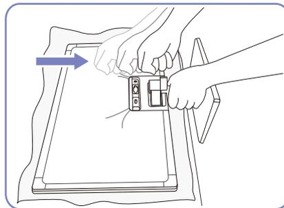
While holding the stand neck with one hand, pound the other fist down onto the top of the stand base in the direction of the arrow to detach the stand base.
