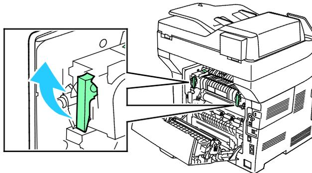
3. Locate the two gray Fuser switches, then slide each one to the setting for envelopes.
