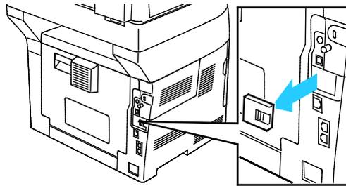
3. Remove the packaging from the Wireless Network Adapter.
