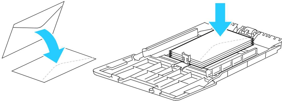
**Note:** When you load Monarch or DL envelopes, remove the Bypass Tray. For details, refer to [Loading Small Paper Sizes in the Bypass Tray](#) on page 150.
