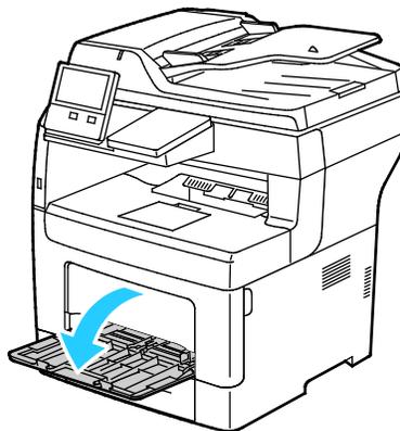
2. To remove the bypass tray from the printer, pull the tray straight out of the printer.
