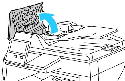
2. With a clean, lint-free cloth that is moistened with water, wipe the feed rollers and the separation pad until they are clean.
