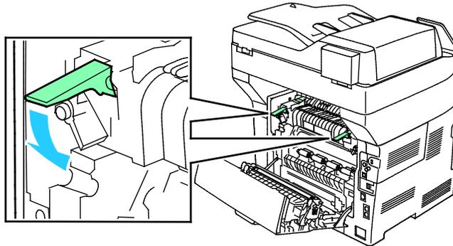
7. Remove any jammed paper from the back of the printer.
