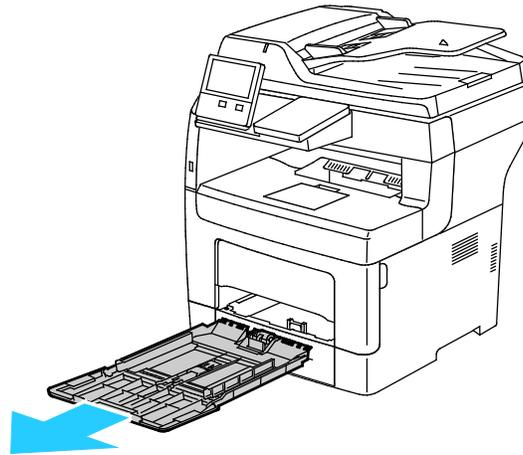
3. If the bypass tray is loaded with paper already, remove any paper that is a different size or type. Raise the paper stop.
