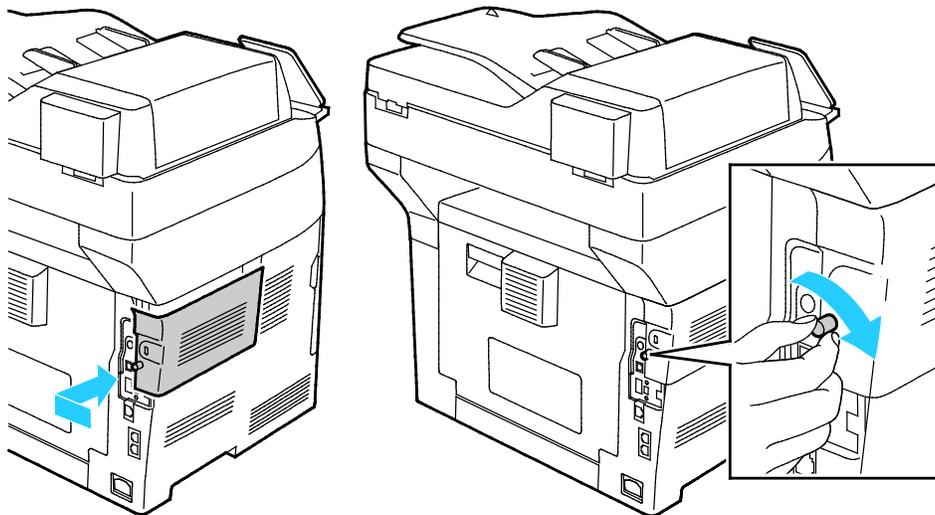
6. Connect the printer to your computer with a USB cable or through the network using an Ethernet cable.
