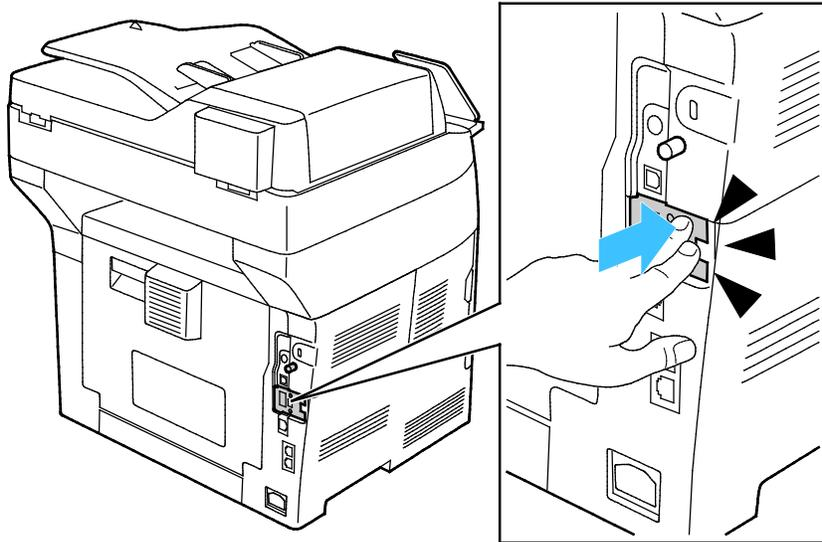
5. Place the left-side cover into position and slide it toward the front of the printer. Tighten the bolt to secure the cover.
