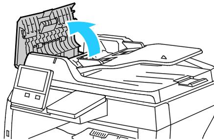
2. If paper is jammed in the Duplex Automatic Document Feeder, open the Document Cover, then remove any jammed paper.
