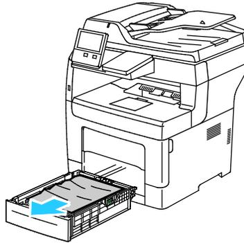
5. Remove any crumpled paper from the tray and any remaining paper jammed in the printer.
