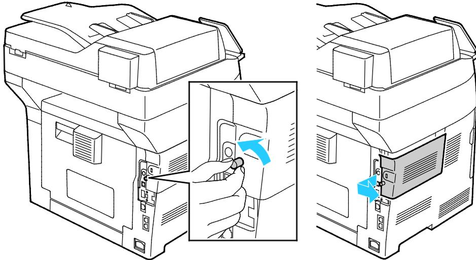
3. Reach into the printer and pull the release lever. Grasp the Wireless Network Adapter with your other hand and carefully pull it away from the printer.
