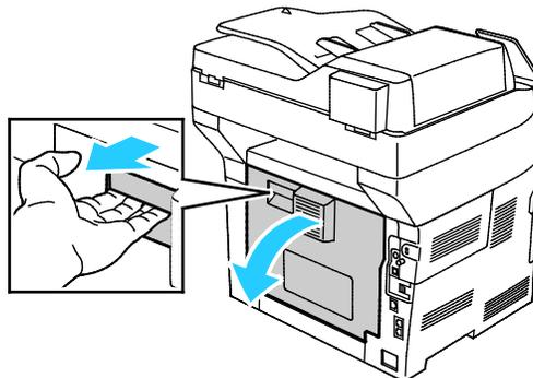
2. If paper is jammed in the Fuser, raise both green levers to open the Fuser.
