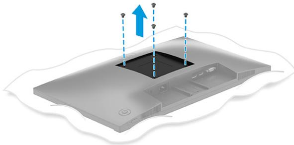
3. To attach the monitor head to a swing arm or other mounting device, insert four mounting screws through the holes on the mounting device and into the VESA screw holes on the back of the monitor head.
