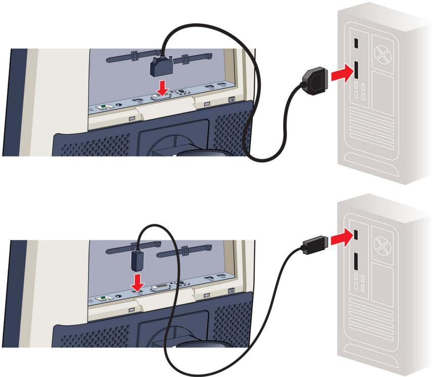
2. If you want to make use of the display's USB upstream connector, connect a PC USB downstream connector to the display's USB upstream connector.
