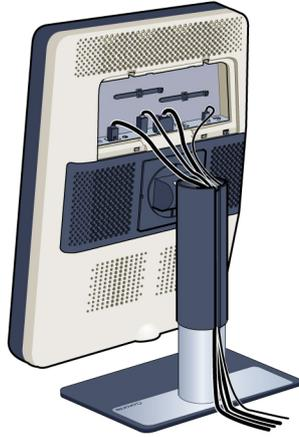
**Tip:** The cable straps at the inside of the connector compartment allow you to fix the cables for better shielding of the cables.
