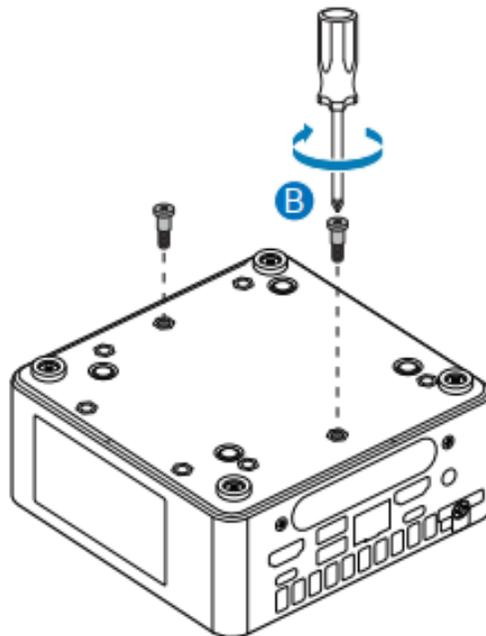
2. Attach the two slightly larger black screws to the bottom chassis cover of the Intel NUC.
