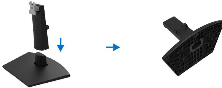
**Figure 10. Assemble the stand**
