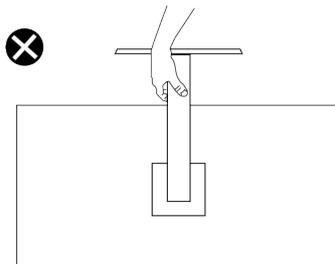
**Figure 9. Do not turn the monitor upside down**
