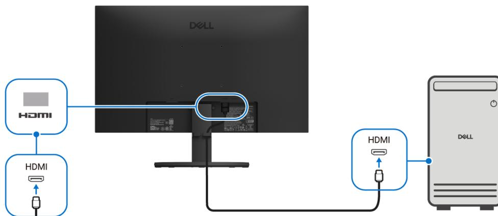
Figure 14. Connecting HDMI cable
