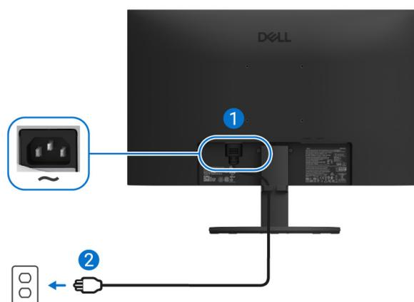
Figure 15. Connecting power cable
