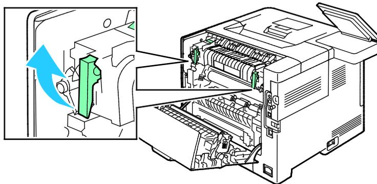
3. Locate the two gray Fuser switches, then slide each one to the setting for envelopes.
