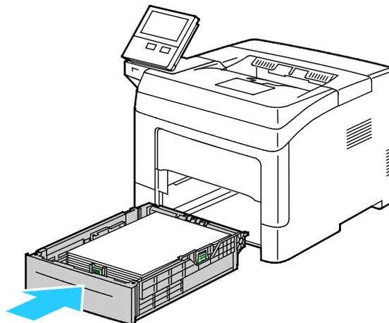
**Note:** If the tray is extended for legal-size paper, the tray protrudes when it is inserted into the printer.
