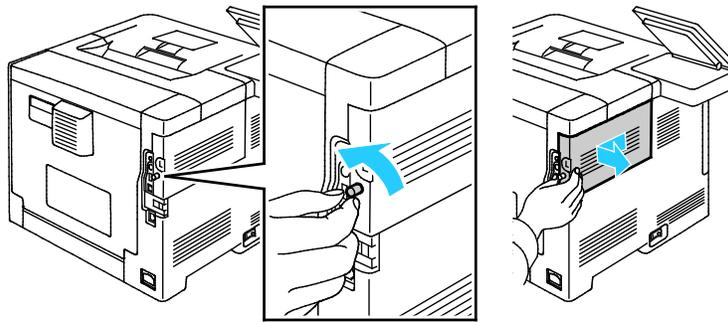
3. To remove the Wireless Network Adapter Port Cover, press the latch to the left, then pull the cover away from the printer.
