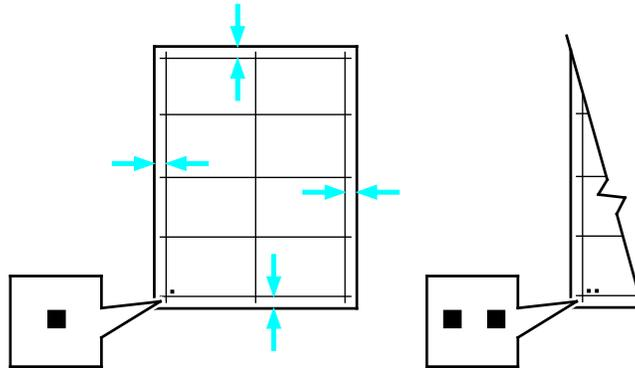
10. For Side 2, measure the distance of the printed image from the top, bottom, left, and right edges.
