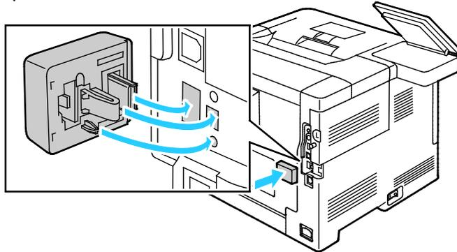
**CAUTION:** Pulling on the adapter can cause damage. After the adapter is installed, remove it only as needed, and as directed in the Wireless Network Adapter removal instructions. For details, refer to Removing the Wireless Network Adapter.
