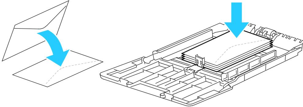
**Note:** Do not load paper above the maximum fill line. Overfilling the tray can cause the printer to jam.
