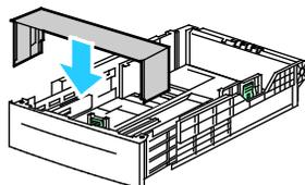
**Note:** If the tray is extended for Legal-size paper, the tray protrudes when it is inserted into the printer.
