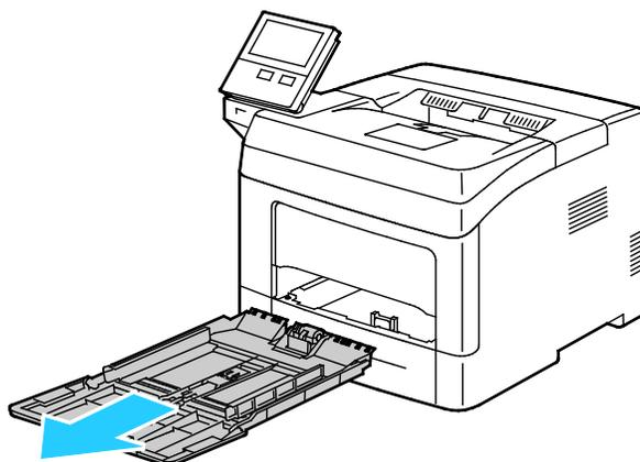
3. If the bypass tray is loaded with paper already, remove any paper that is a different size or type. Raise the paper stop.
