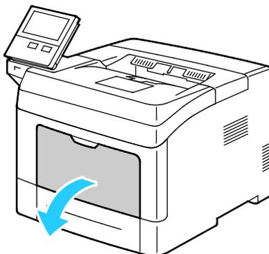
2. To remove the bypass tray from the printer, pull the tray straight out of the printer.
