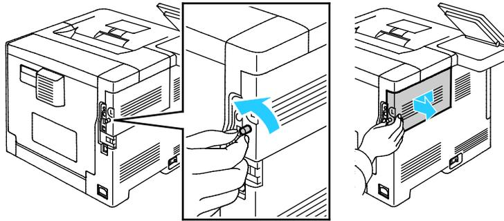
3. Reach into the printer and pull the release lever. Grasp the Wireless Network Adapter with your other hand and carefully pull it away from the printer.
