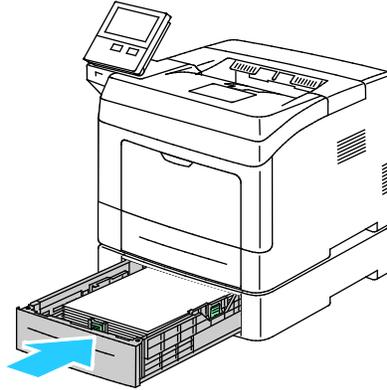
6. Push the tray completely back into the printer.
