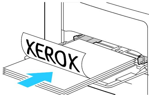
**Note:** Do not load paper above the maximum fill line. Overfilling the tray can cause the printer to jam.
