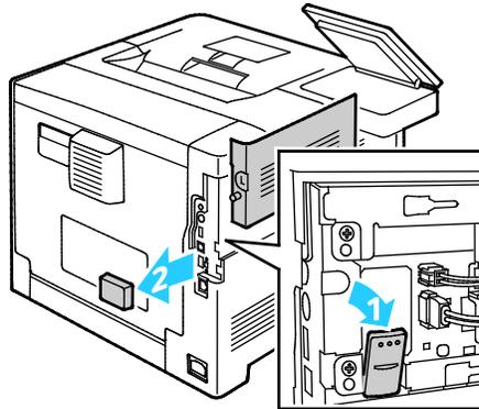
**CAUTION:** Do not use force to pull on the Wireless Network Adapter. If the latch is released properly, the adapter pulls out easily. Pulling on a secured adapter can damage it.
