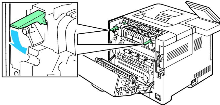
7. Remove any jammed paper from the back of the printer.
