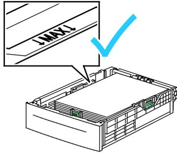
5. Adjust the length and width guides to fit the paper.
