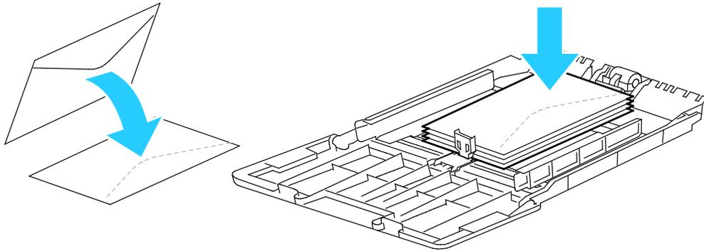
**Note:** When you load Monarch or DL envelopes, remove the Bypass Tray. For details, refer to [Loading Small Paper Sizes in the Bypass Tray](#) on page 107.
