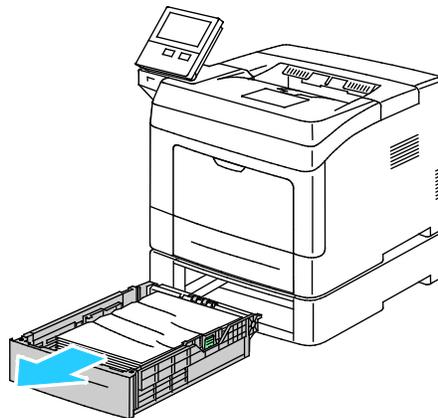
3. Remove any crumpled paper from the tray and any remaining paper jammed at the front of the printer.
