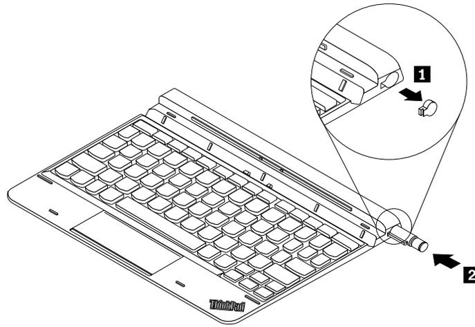
Figure 7. Storing the pen in the keyboard
