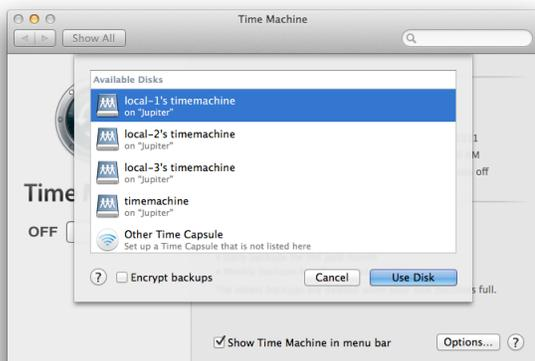
7. Select the disk named *user name timemachine* and click the **Use Disk** button. The connect window opens requesting the user name and password.
