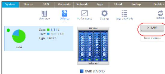
3. Confirm that you want to switch from X-RAID to Flex-RAID. The volume switches from Flex-RAID mode to X-RAID mode and the indicator on the X-RAID button turns green.
