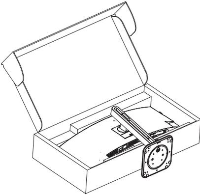
2. While keeping the release button pressed, tilt the base and slide it out.
