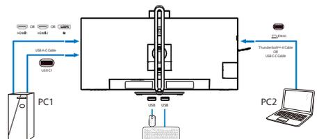
2. Enter the On-Screen Display (OSD) menu. Go to the KVM tab and select "Auto", "Thunderbolt", or "USB C" to switch the monitor view from one device to another. To switch to another monitor view, simply repeat this step.
