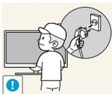
Before moving the product, turn off the power switch and disconnect the power cable and all other connected cables.
