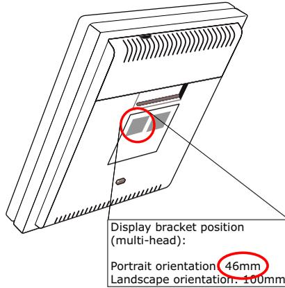
Figure 18: Example of label with position for brackets
