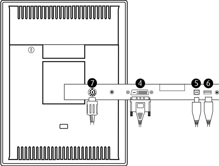
Figure 25: Signal cable connections
