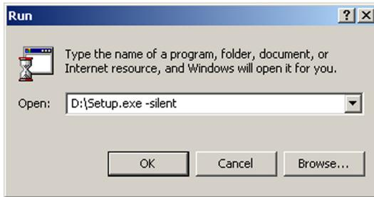
Figure 34: Command line installation
