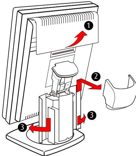
Figure 24: Remove covers before connecting signal cables
