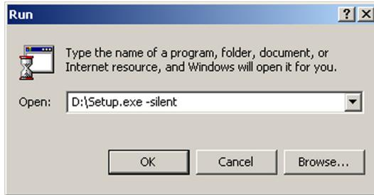
Figure 31: Command line installation
