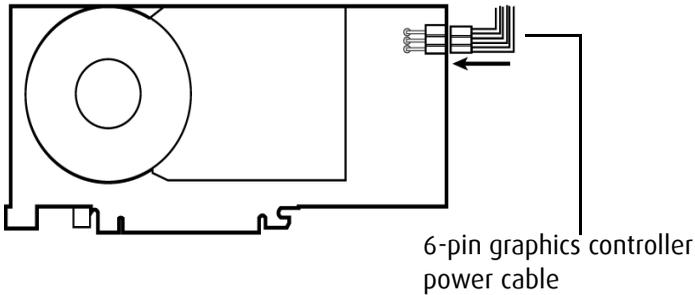
Figure 4: Power connection for the MXRT 5100 and 7100 controllers
