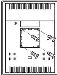
Figure 21: : Vesa mount fixation holes
