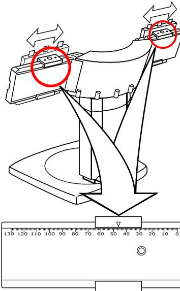
Figure 19: Shift brackets according to label indication
