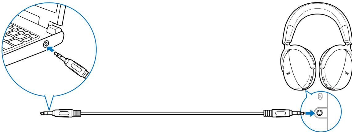
Figure 21. Audio cable connection
