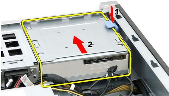
5. Remove the screws from the optical drive and remove the bracket.
