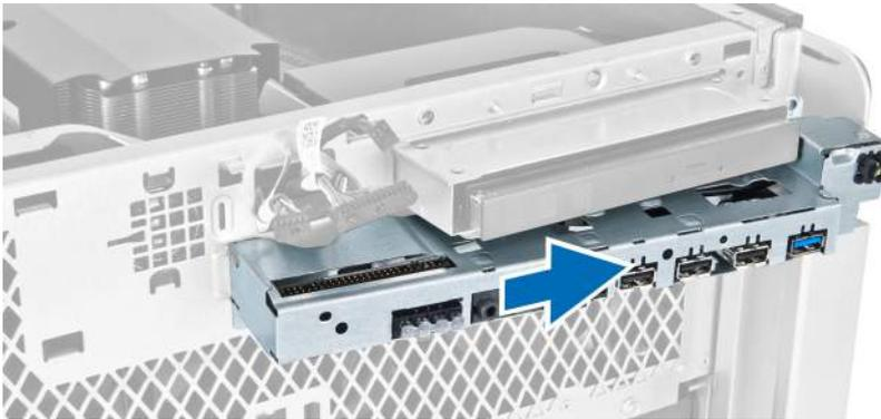
7. Remove the screws that secure the USB 3.0 module to the I/O panel and remove it from the computer.
