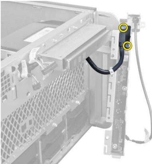
8. Remove the screws that secure the I/O panel and remove it from the computer.
