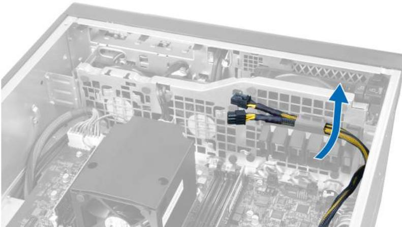
7. Pull the second air duct in the direction opposite to the system fan module.
