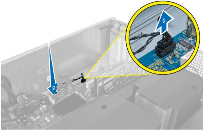
4. Unroute the thermal-sensor cable from its securing clips on the chassis.
