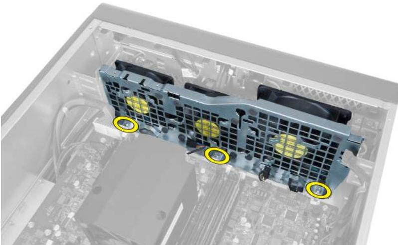
12. Insert the fan cable through the opening to release the system-fan module.
