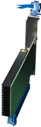
4. Press down the latch and pull the PCI card away from the computer.
