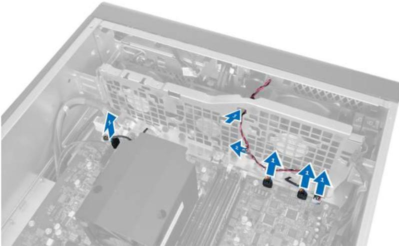
11. Remove the screws that secure the system-fan module to the chassis.
