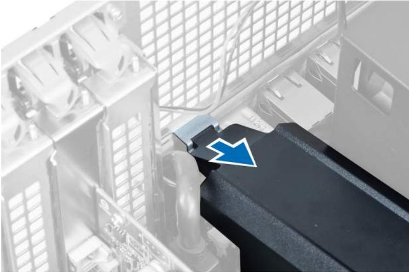
5. Press down on the release latch on the air tunnel base and lift it upwards to remove it from the computer.
