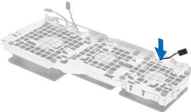
13. Remove the grommets that secure the system fan , lift up the fan and remove it from the fan assembly.
