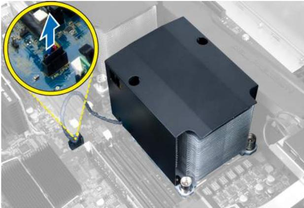
4. Remove the captive screws that secure the heatsink.
