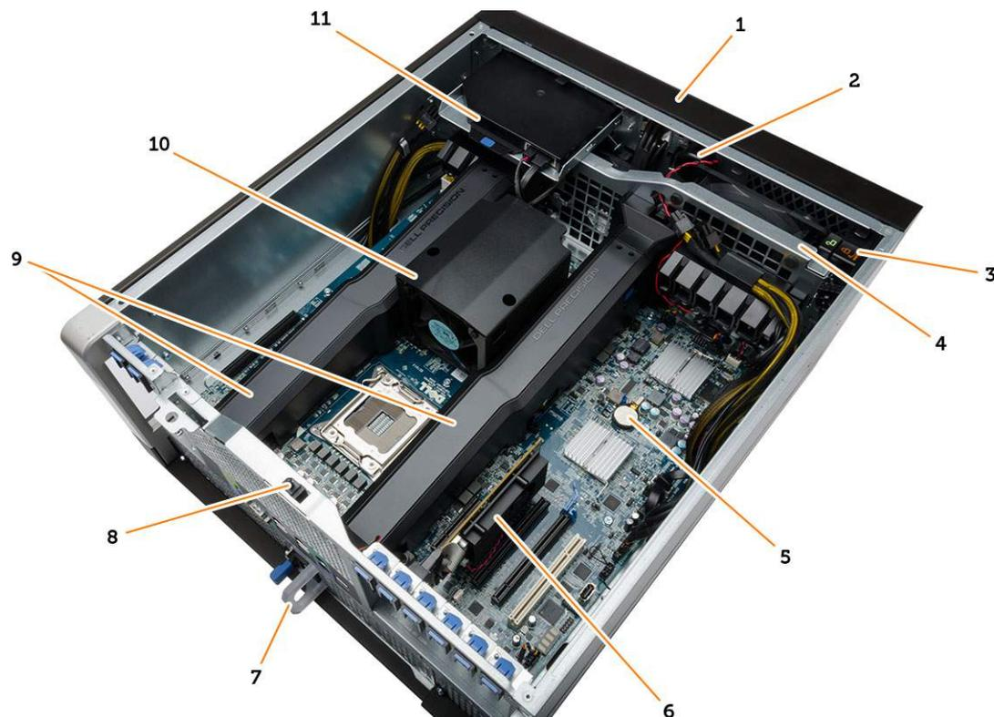
**Figure 1. Inside View of the T7610 Computer**
