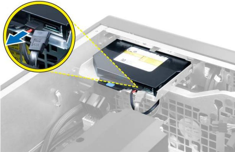
5. Press down on the blue release tab to release the latches that secure the optical drive.
