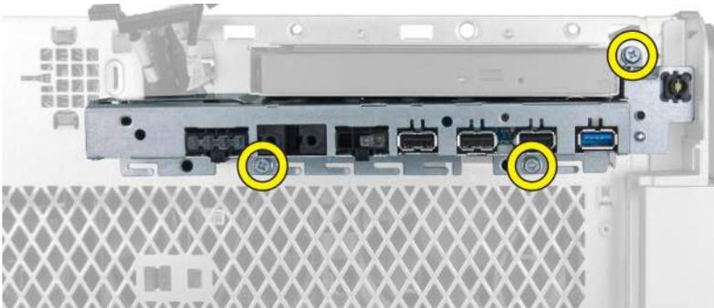
5. Pull the I/O panel in a direction opposite to the computer to release its edge from the chassis clip.
