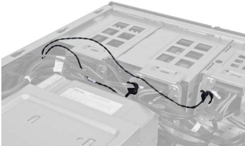
5. Open the latch securing the thermal sensor and remove it from the computer.
