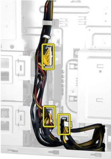
4. Remove the screws that secure the PSU card to the chassis and remove it from the computer.
