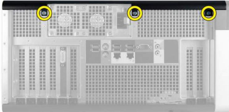
3. Slide the right cover in the direction indicated to remove it from the computer.
