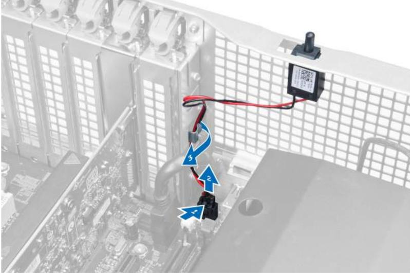
4. Push the intrusion switch downwards and remove it from the computer.
