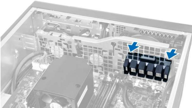
8. Lift the second air duct in an upwards direction to remove it from the computer.
