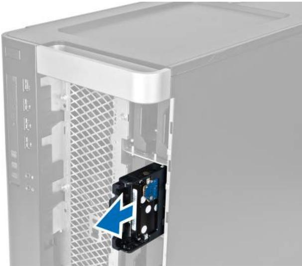
7. Flex the hard-drive bracket on both sides to loosen the hard drive.
