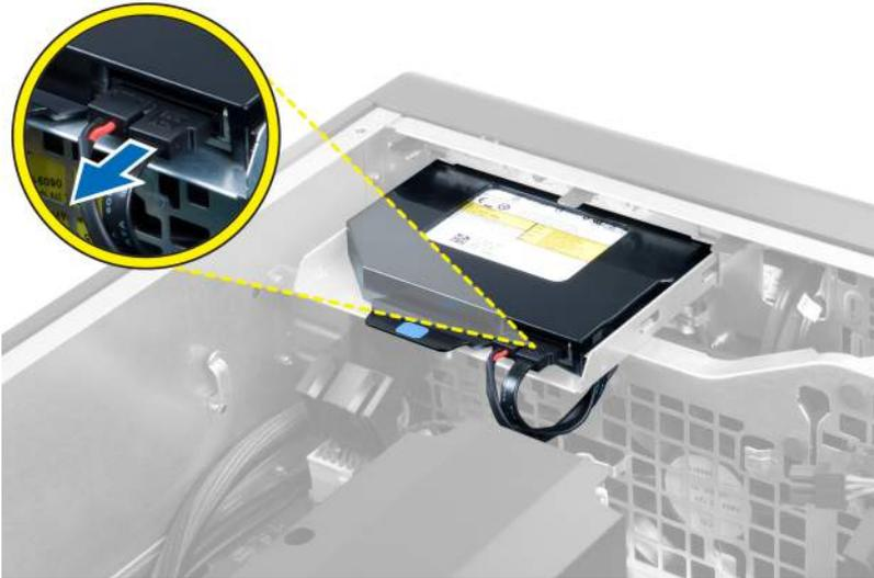
4. Disconnect the power cable from the back of the optical drive.
