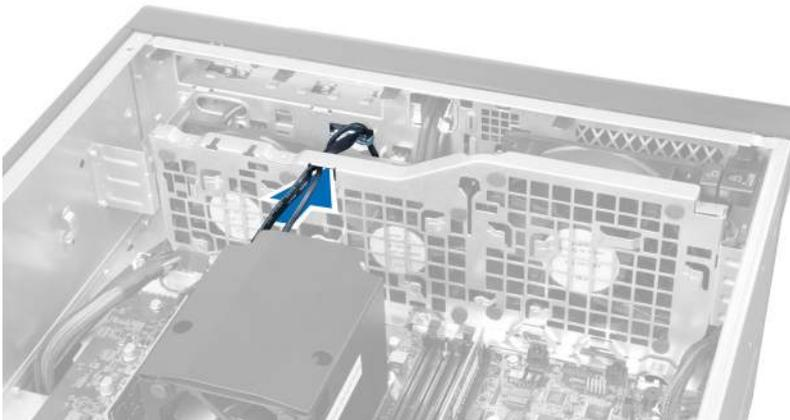
10. Disconnect the system-fan cable connectors from the system board.
