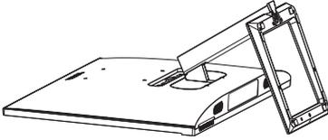
2. Use screwdriver to loosen the screw located at the bottom of the base, and remove the base from the stand.
