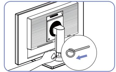
You can remove the fixing pin and adjust the stand now.
