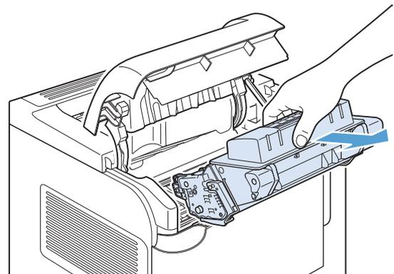
3. Use the green handle to lift the paper-access plate. Slowly pull the jammed paper out of the product. Do not tear the paper. If paper is difficult to remove, try clearing it from the tray area.
