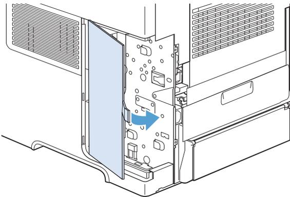
7. Reinstall the right-side panel. Align the tabs on the panel with the slots in the product, and push the panel toward the front of the product until it latches into place.
