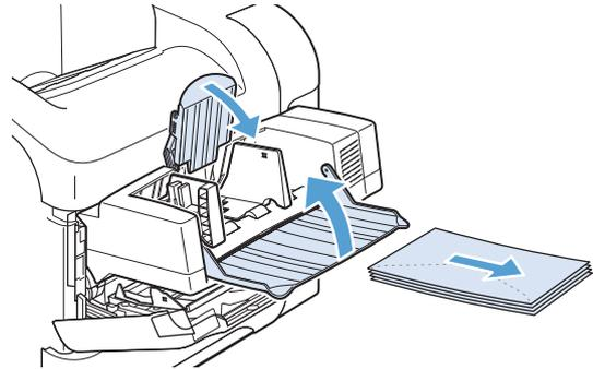
2. Grasp both sides of the optional envelope feeder and carefully pull it out of the product.
