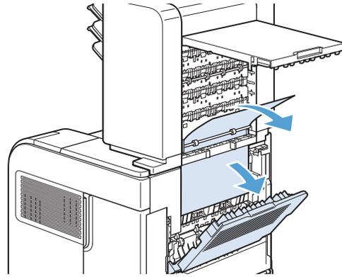
5. Close the jam-access door and the rear output bin.
