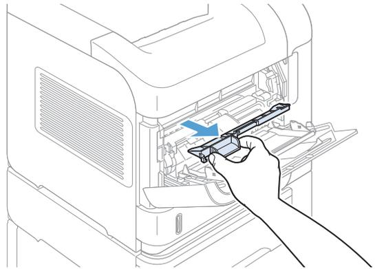
5. Rotate the paper guide to check for additional jammed paper underneath. If jammed paper is present, remove it.
