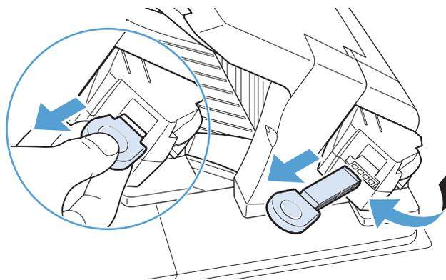
2. Rotate the green cover on the end of the staple cartridge upward, and remove the jammed staple.
