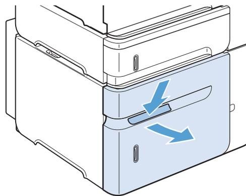
2. If the edge of the jammed paper is visible in the feed area, slowly pull the paper down and out of the product. (Do not pull the paper straight out, or it will tear.) If the paper is not visible, look in the top-cover area.
