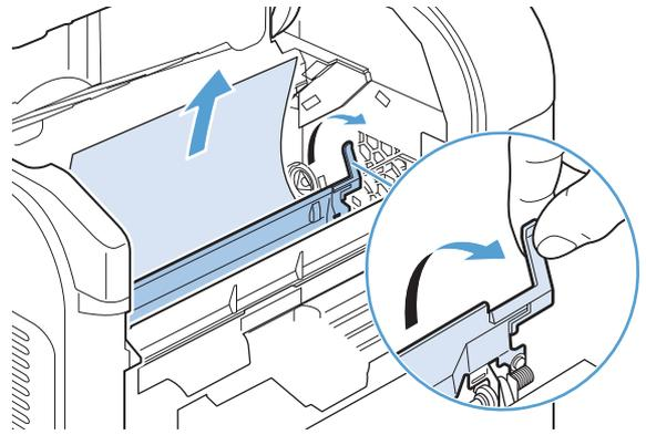
4. Open Tray 1 and remove the envelope accessory cover. If paper is present, remove it.
