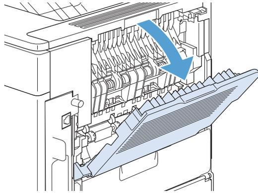
5. Remove the rear output bin. Place your finger near the left-side hinge, and push firmly to the right until the hinge-pin clears the hole inside the product. Rotate the output bin outward to remove it.
