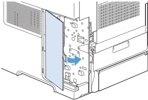
10. Reinstall the right-side panel. Align the tabs on the panel with the slots in the product, and push the panel toward the front of the product until it latches into place.
