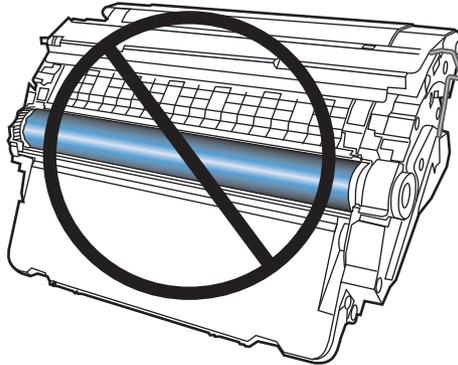
4. If you see any scratches, fingerprints, or other damage on the imaging drum, replace the print cartridge.
