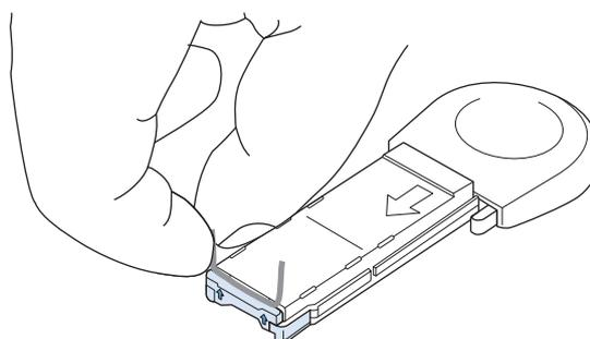
3. Insert the staple cartridge into the stapler unit, and rotate the stapler unit toward the rear of the product until the unit snaps into place.
