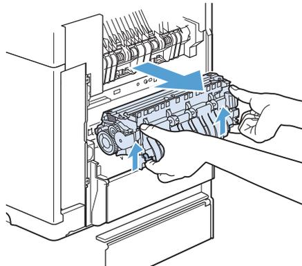
7. Remove the jammed paper. If necessary, lift the black plastic guide that is located on the top of the fuser to gain access to the jammed sheet.
