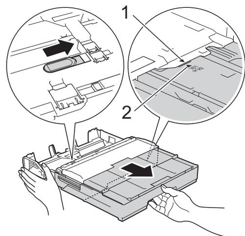
Push the blue slider a second time until it locks in the release position, and then extend the tray until the blue slider returns to and locks in the default position. Open the tray cover and make sure the triangular mark inside the tray (1) lines up with the mark (2) for **A3/LGR**, as shown in the illustration.
