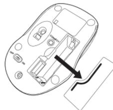
2. Insert the two AAA batteries, making sure that the positive (+) and negative (-) ends of each battery match the polarity indicators inside the battery compartment.
