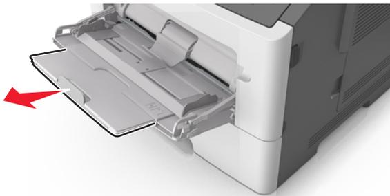
**b** Pull the extender gently so that the multipurpose feeder is fully extended and open.
