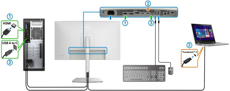
**NOTE:** The USB-C connection currently supports video and data transfer. Ensure **USB Selection** for **HDMI** is set to **USB-C**.
