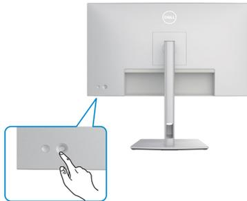
To modify the OSD adjustments using the joystick control on the rear end of the monitor, do the following:
