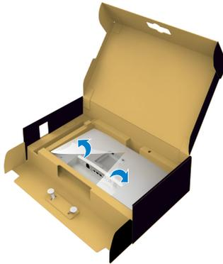
6. Carefully insert the tabs on the stand riser into the slots on the display back-cover and press down the stand assembly to snap it into place.
