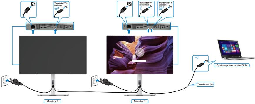
Similarly, a PC is connected to two monitors in an initially ON power state, and the PC system power state is in sync with Monitor 1 power button. When you press the Monitor 1 or PC power button, both the Monitor 1 and PC turns OFF. Meanwhile the Monitor 2 will be in Standby mode. You need to manually press the power button on Monitor 2 to turn it OFF.
