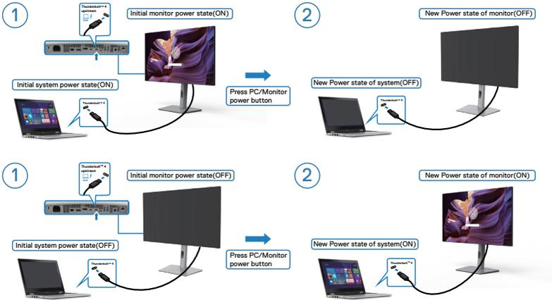
When the monitor and PC power state are both ON, while you **press and hold 4 seconds on monitor power button**, the screen prompt will ask if you would like to shut down the PC.
