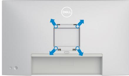
**NOTE: Use M4 x 11 mm screws to connect the monitor to the wall-mounting kit.**
