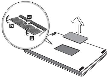
4. Replace the memory cover and secure it with the screw.
