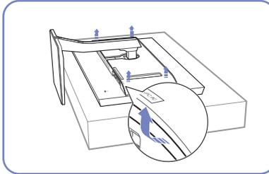
Remove the rear cover by pulling the corners in the direction of the arrows.
