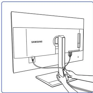
Hold the bottom of the stand neck securely with your left hand and use the thumb of your right hand to slide up the COVER-CABLE to fix it in place.
