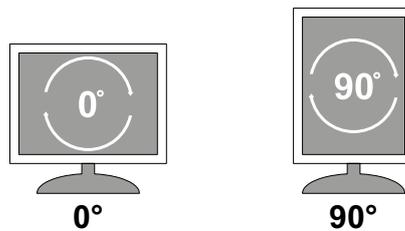
The on-screen display (OSD) menu items will automatically rotate when the screen rotates.
