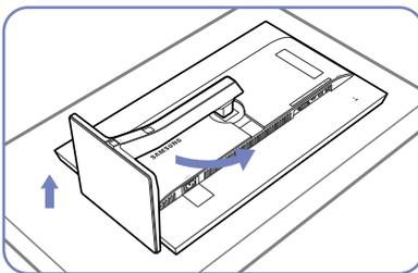
Place a protective cloth or cushion on a flat surface. Next, place the product with the face down on top of the cloth or cushion. Rotate the stand body about 90°.
