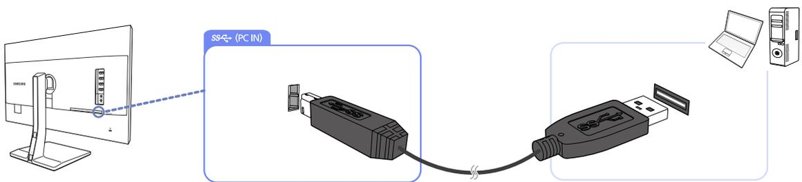
Connect the USB cable to [
