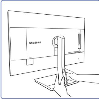
Remove the COVER-CABLE by sliding it down with both hands in the direction indicated by the arrow.
