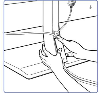
Hold the COVER-CABLE and fix the cables into the grooves on the STAND-REAR.
