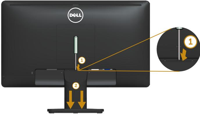
After placing the monitor panel on a soft cloth or cushion, complete the following steps to remove the base:
