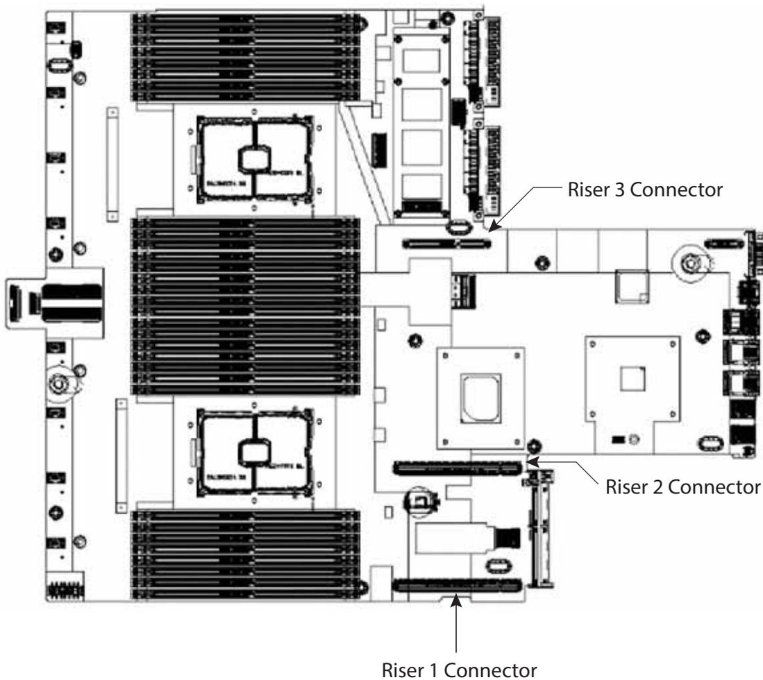
Figure 10 shows three half-height risers plugged into their respective connectors.
