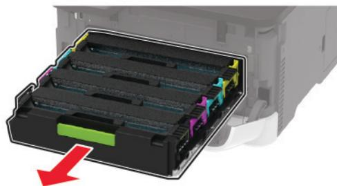
**3** Remove the used print cartridge.
