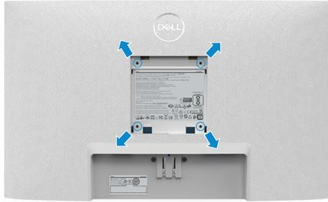
**NOTE:** Use M4 x 10 mm screws to secure the wall-mounting kit to the monitor.
