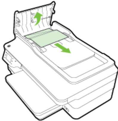
2. Lift the tab located on the front edge of the ADF.
