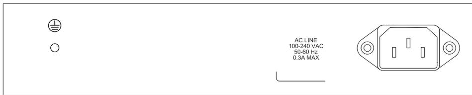
Figure 1-13. Rear panel view of the DES-3200-18 Ver. A1
