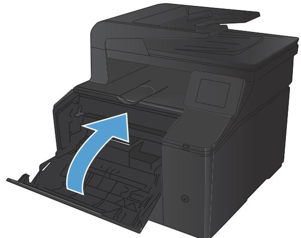
12. Place the old toner cartridge and the plastic shield in the box for the new toner cartridge. Follow the recycling instructions that are included in the box.
