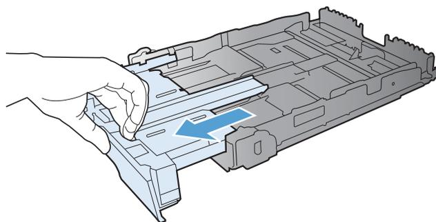
4. Place the paper in the tray and make sure that it is flat at all four corners. Slide the paper length and width guides so that they are against the stack of paper.
