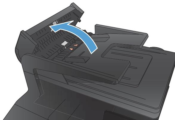
3. Lift the document feeder roller assembly, and gently pull the jammed paper out.
