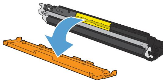
7. Do not touch the imaging drum on the bottom of the toner cartridge. Fingerprints on the imaging drum can cause print-quality problems.
