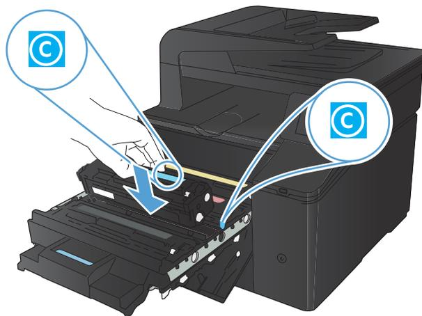
9. Pull the tab on the left side of the toner cartridge straight up to completely remove the sealing tape. Discard the sealing tape.
