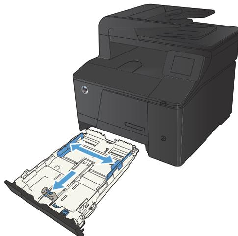
3. To load Legal-size paper, extend the tray by pressing and holding the extension tab while pulling the front of the tray outward.
