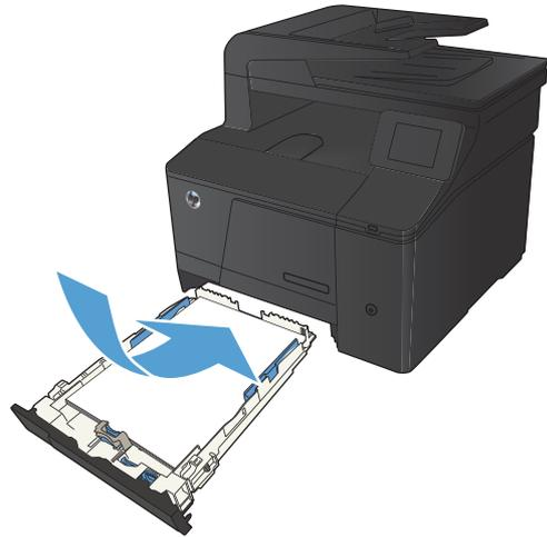
5. Push down on the paper to make sure that the paper stack is below the paper limit tabs on the side of the tray.
