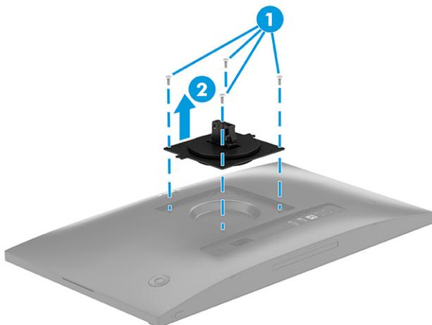
4. To attach the monitor head to a swing arm or other mounting device, insert four mounting screws through the holes on the mounting device and into the VESA screw holes on the back of the monitor head.
