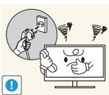
If the product generates a strange noise, a burning smell, or smoke, remove the power cord immediately and contact Samsung Customer Service Center (page 95).
