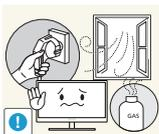
If a gas leakage is found, do not touch the product or power plug. Also, ventilate the area immediately.
