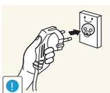
Ensure you connect the power plug to a grounded power socket. (type 1 insulated devices only).
