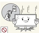
If the product falls or the exterior is damaged, power off the product, remove the power cord, and contact Samsung Customer Service Center (page 95).
