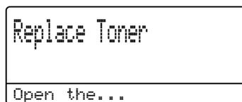
The machine will stop printing until you replace the toner cartridge. A new genuine Brother toner cartridge will reset the `Replace Toner` mode.
