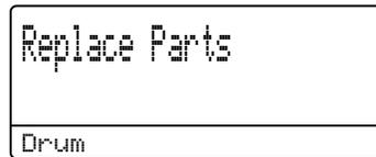
The drum unit has exceeded its rated life. Please replace the drum unit with a new one. We recommend a genuine Brother drum unit be installed at this time.
