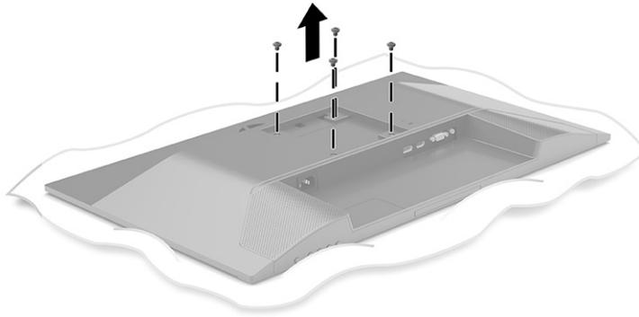
2. To attach the monitor head to a swing arm or other mounting device, insert four mounting screws through the holes on the mounting device and into the VESA screw holes on the back of the monitor head.
