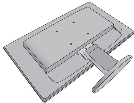
Detach the monitor base as instructed in [How to detach the base on page 13](#).
