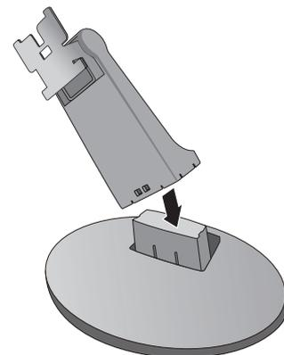
Orient and align the stand arm with the monitor, then push them together until they click and lock into place.
