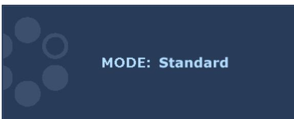
Press the ▼ key continually to switch between the 6 modes for the main window, including **Standard**, **Movie**, **Game**, **Photo**, **sRGB**, and **Eco**. The setting will take effect immediately.
