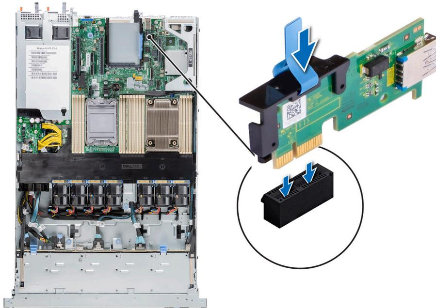
**Figure 91. Installing the internal USB card**
