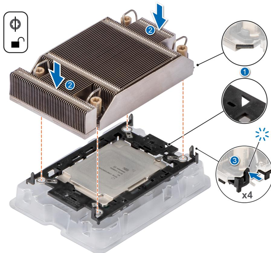
Figure 54. Installing the heat sink onto the processor
