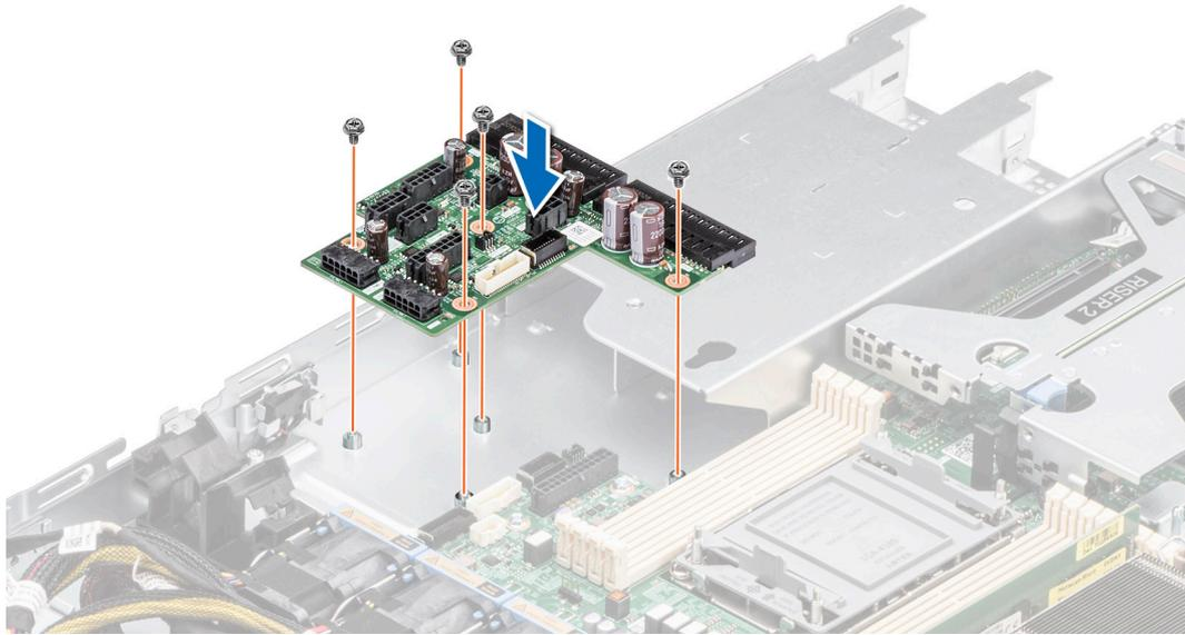
**Figure 99. Installing the power interposer board**
