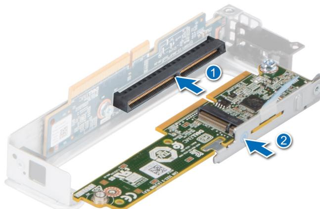
**Figure 79. Installing the M2 BOSS card into the M.2 BOSS riser**
