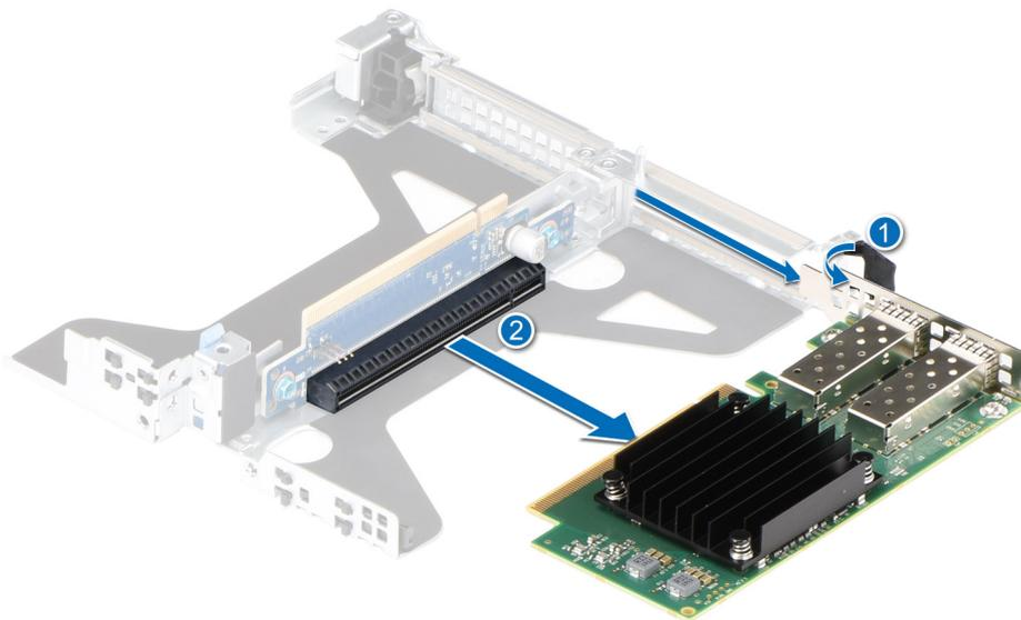
**Figure 65. Removing an expansion card from Riser 2c**
