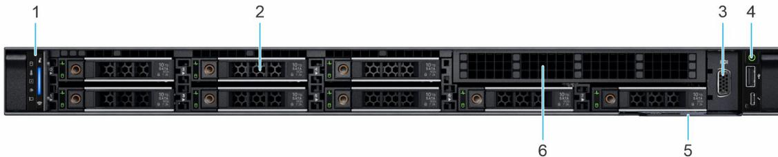
**Figure 2. Front view of 8 x 2.5-inch drive system**
