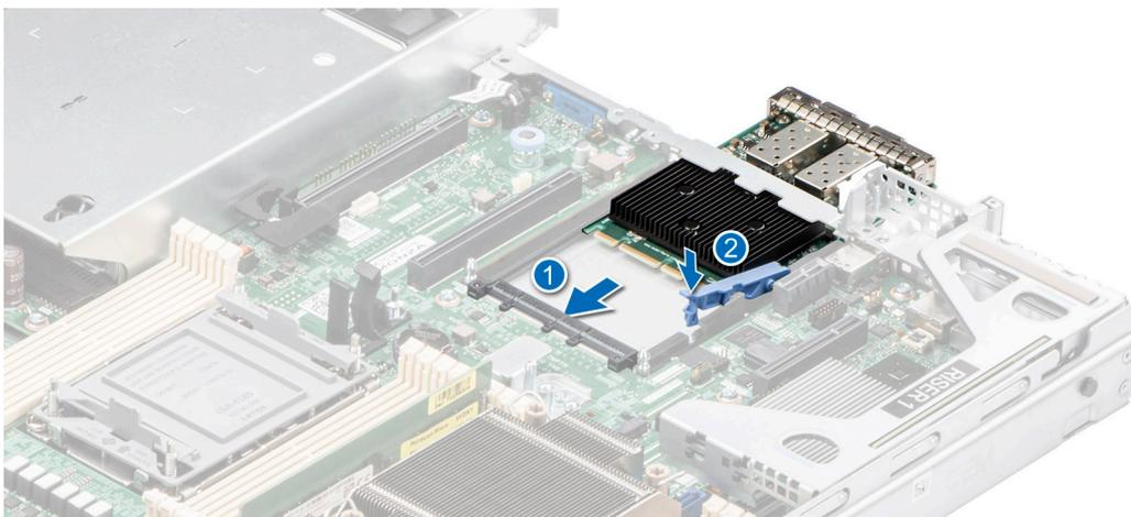
**Figure 83. Installing the OCP card**
