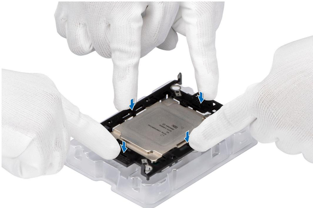
**Figure 51. Press the carrier on the four sides**
