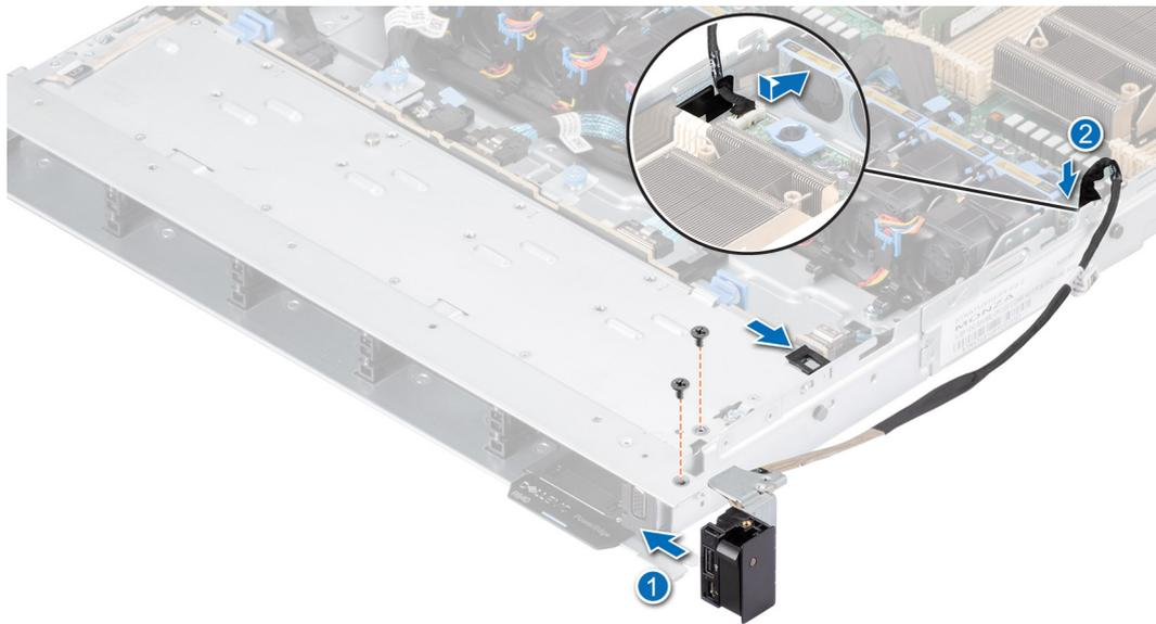
**Figure 106. Installing the right control panel**
