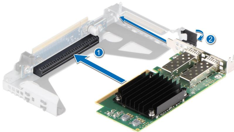
**Figure 70. Installing an expansion card into a Riser 1**
