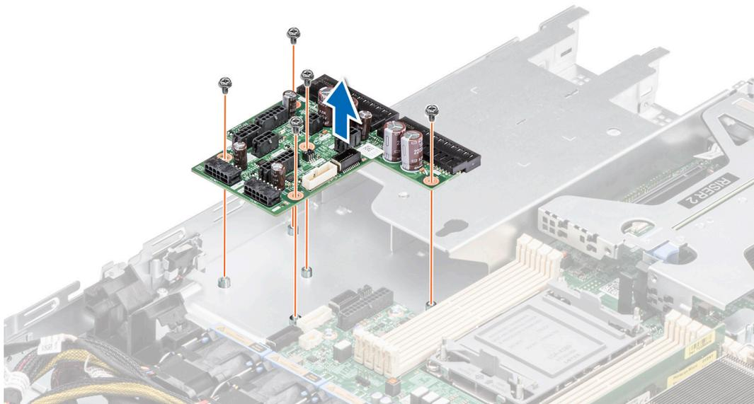
**Figure 98. Removing the power interposer board**
