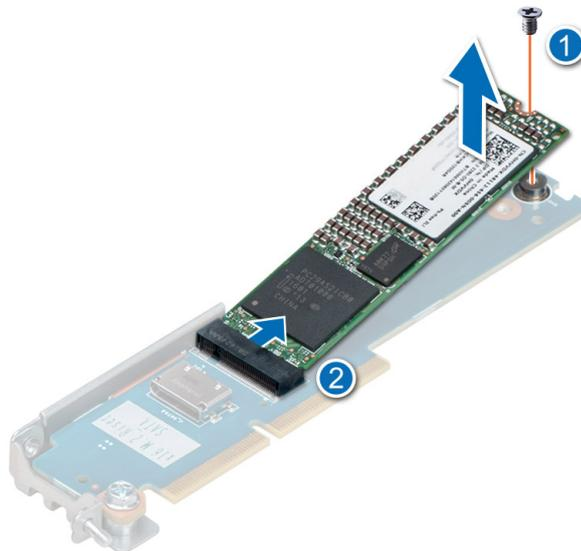
**Figure 80. Removing the M.2 SSD module**
