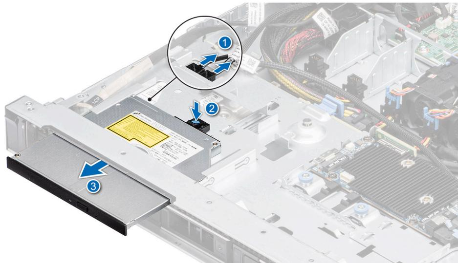
**Figure 33. Removing the optical drive**
