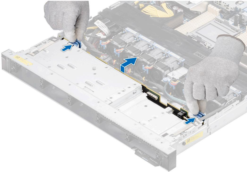
**Figure 37. Removing the backplane**
