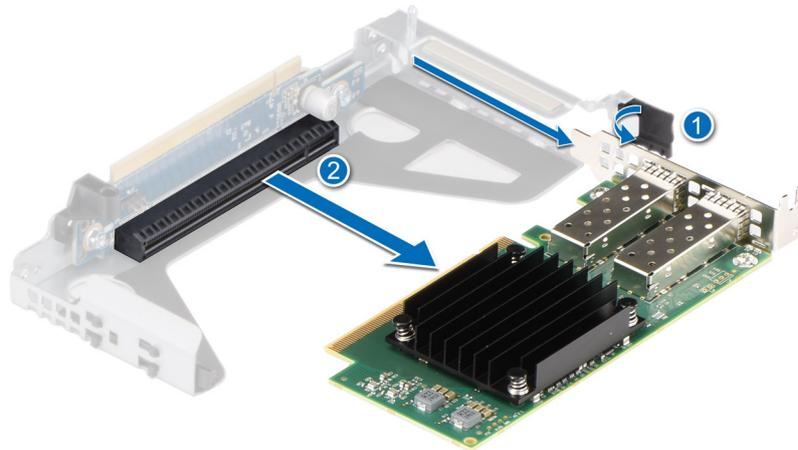
Figure 64. Removing an expansion card from the Riser 1
