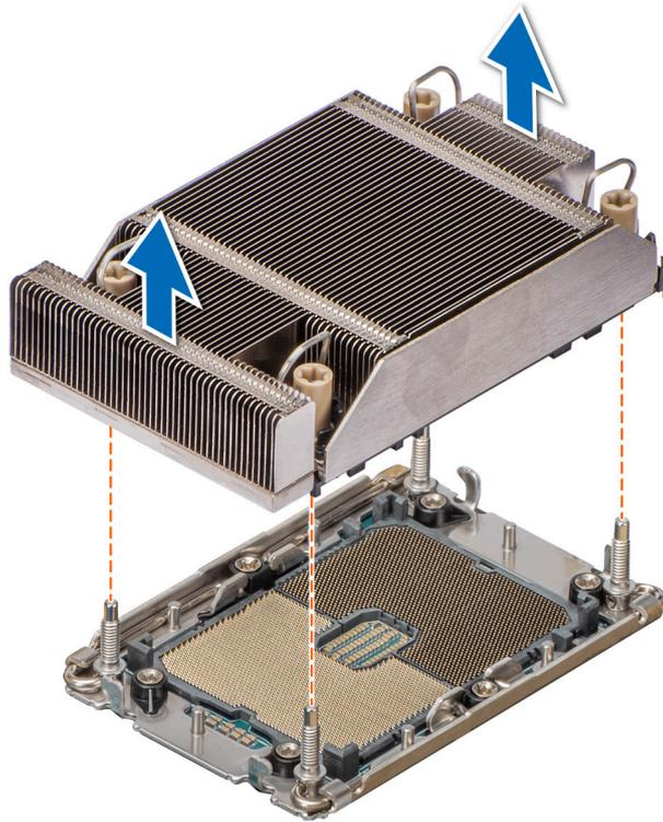
Figure 46. Removing a processor and heat sink module
