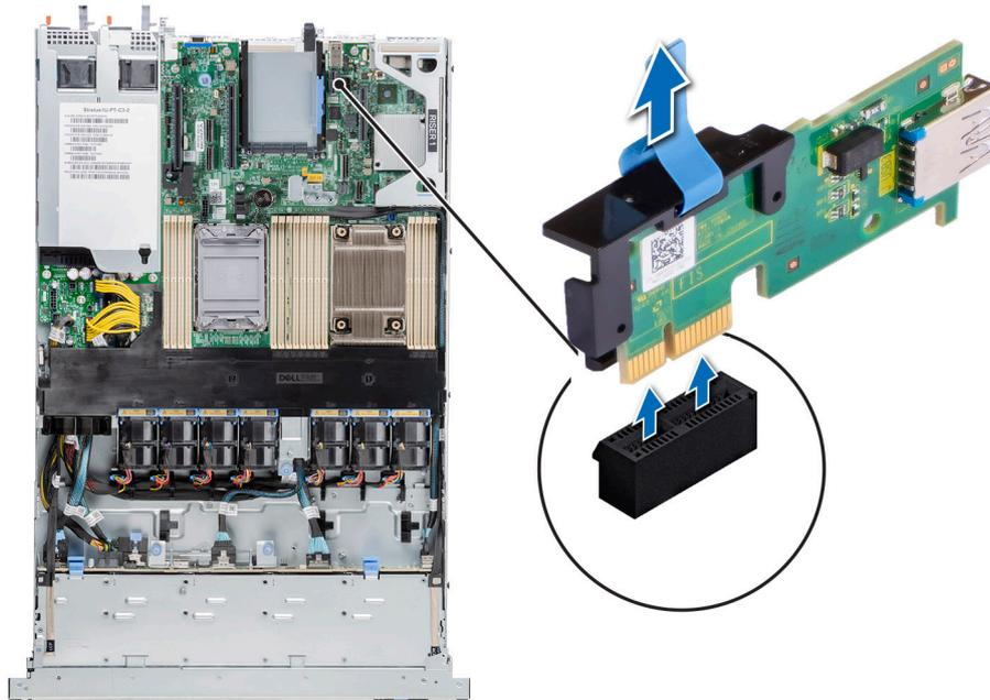
**Figure 90. Removing the internal USB card**
