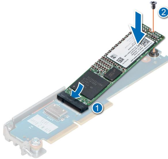
**Figure 81. Installing the M.2 SSD module**
