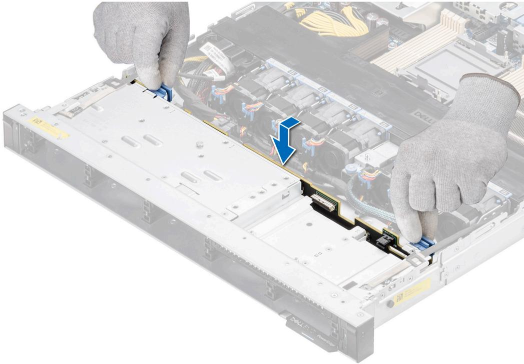
**Figure 38. Installing the drive backplane**
