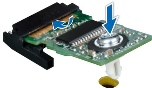
Figure 102. Installing the TPM
