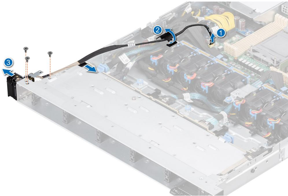
**Figure 103. Removing the left control panel**
