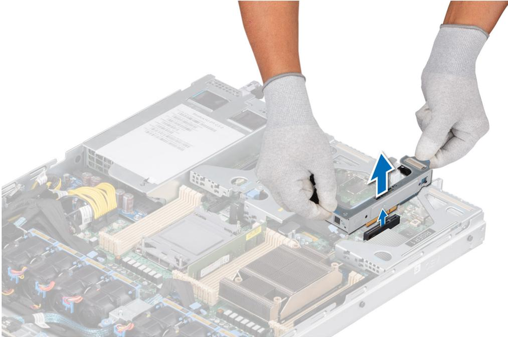
Figure 76. Removing the M.2 BOSS riser
