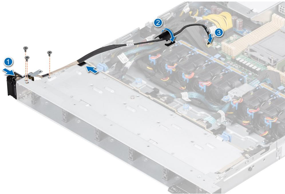
**Figure 104. Installing the left control panel**
