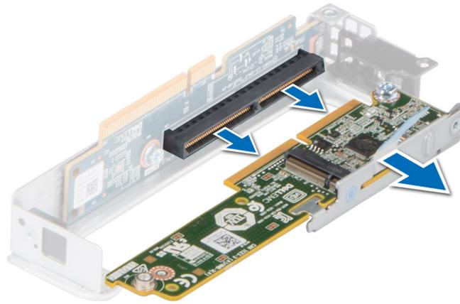
**Figure 78. Removing the M.2 BOSS card from the M.2 BOSS riser**
