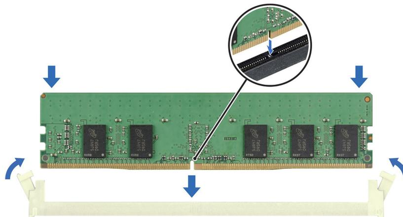
Figure 44. Installing a memory module
