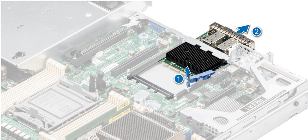
**Figure 82. Removing the OCP card**
