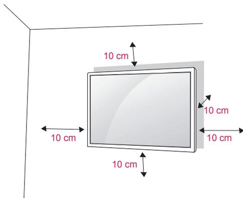
If you intend to mount the Monitor to a wall, attach Wall mounting interface (optional parts) to the back of the set.
