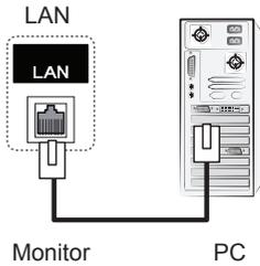
B Using a router(Switch)
