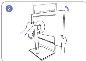
Rotate the machine to the highest vertical position.
