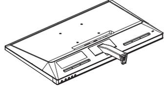
2. Hold the base stand with both hands and firmly insert the base stand into the base column.
