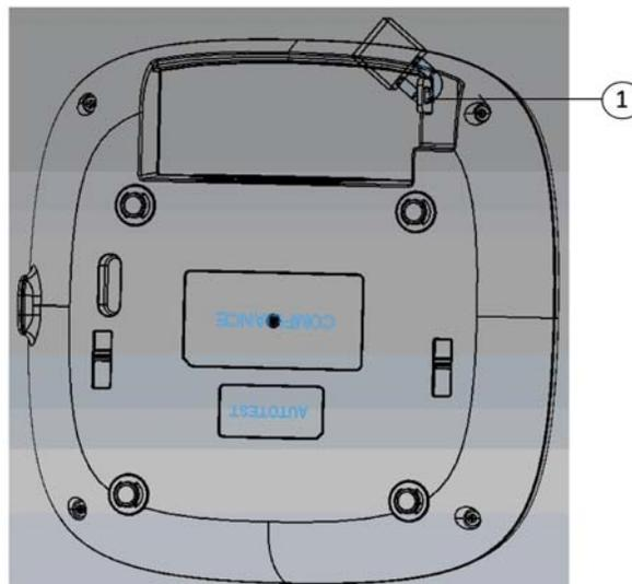
**1** Position of the hasps for the locks on the back of the 9115AXI and 9115AXE models
