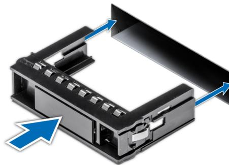
Figure 25. Installing a drive blank
