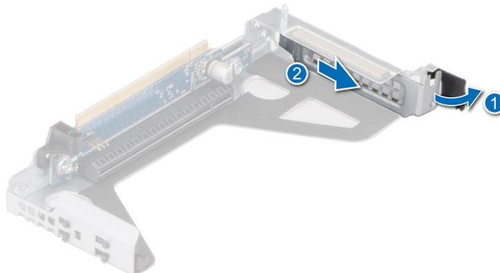
**Figure 85. Removing a filler bracket from Riser 1**
