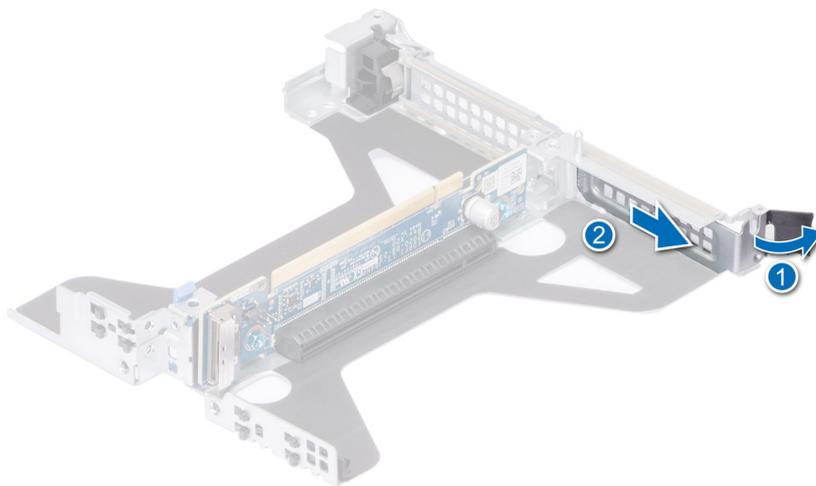
Figure 87. Removing filler bracket from Riser 2b (SNAPI)
