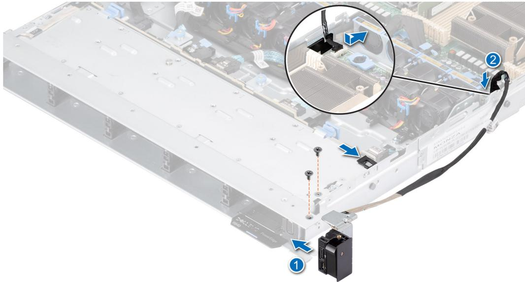
**Figure 131. Installing the right control panel**
