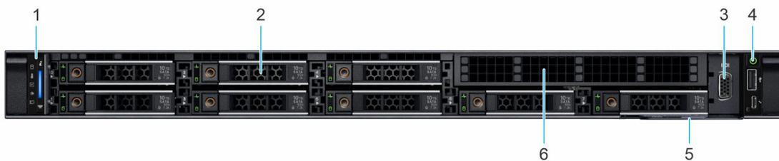
**Figure 2. Front view of 8 x 2.5-inch drive system**
