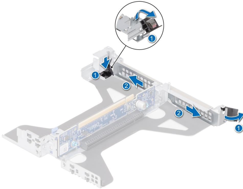
Figure 86. Removing filler bracket from Riser 2a
