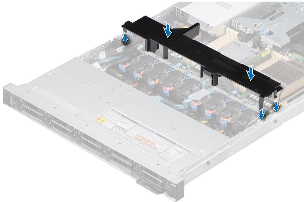
**Figure 19. Installing the air shroud**
