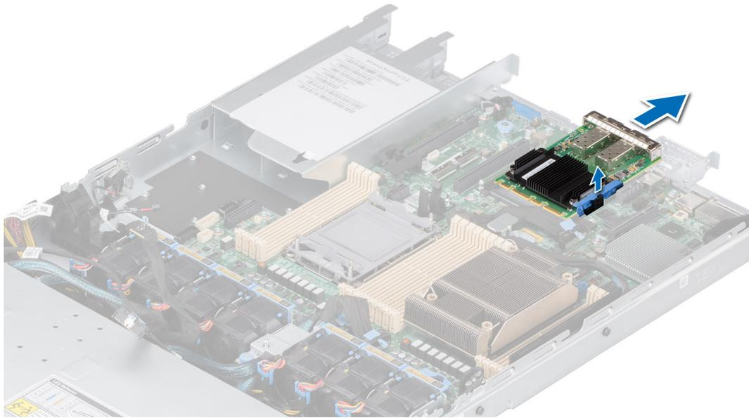
**Figure 109. Removing the OCP card**
