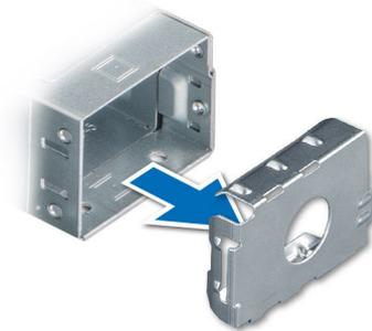
Figure 119. Removing a power supply unit blank
