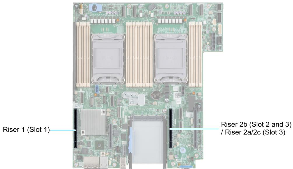
**Figure 64. Expansion card slot connectors**
