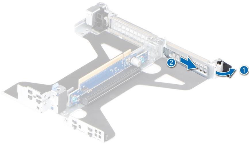
**Figure 88. Removing filler bracket from Riser 2c**
