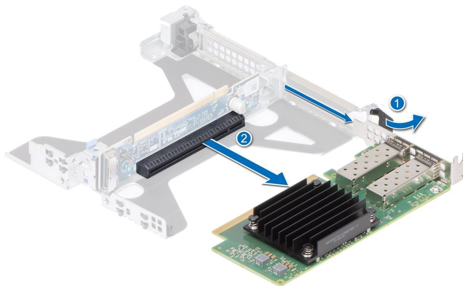
Figure 79. Removing an expansion card from Riser 2b (SNAPI)
