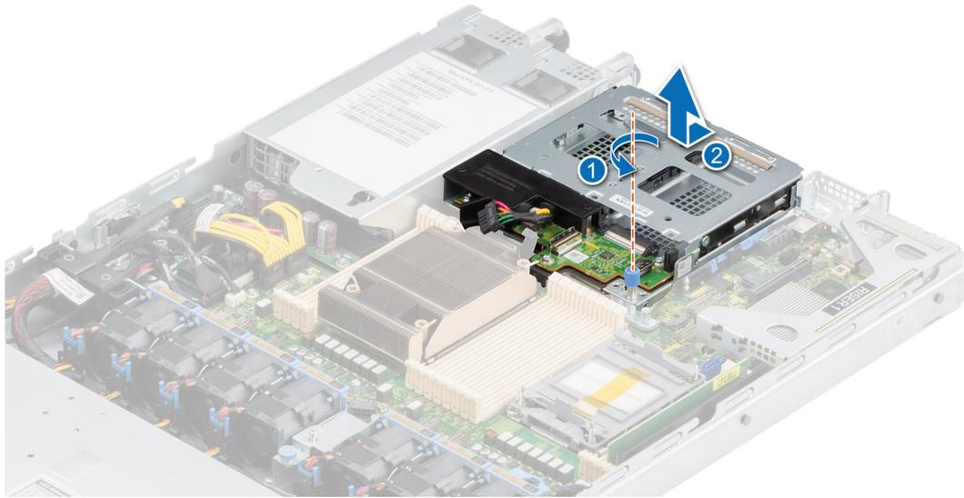
**Figure 93. Removing the 2.5-inch rear drive cage**
