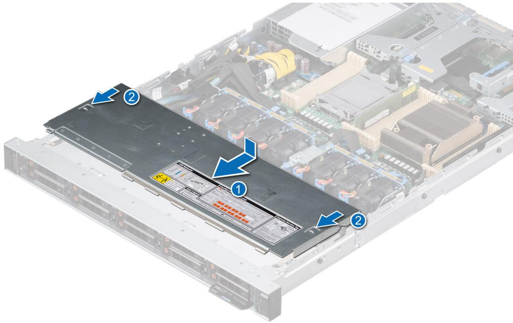
**Figure 17. Installing the drive backplane cover**
