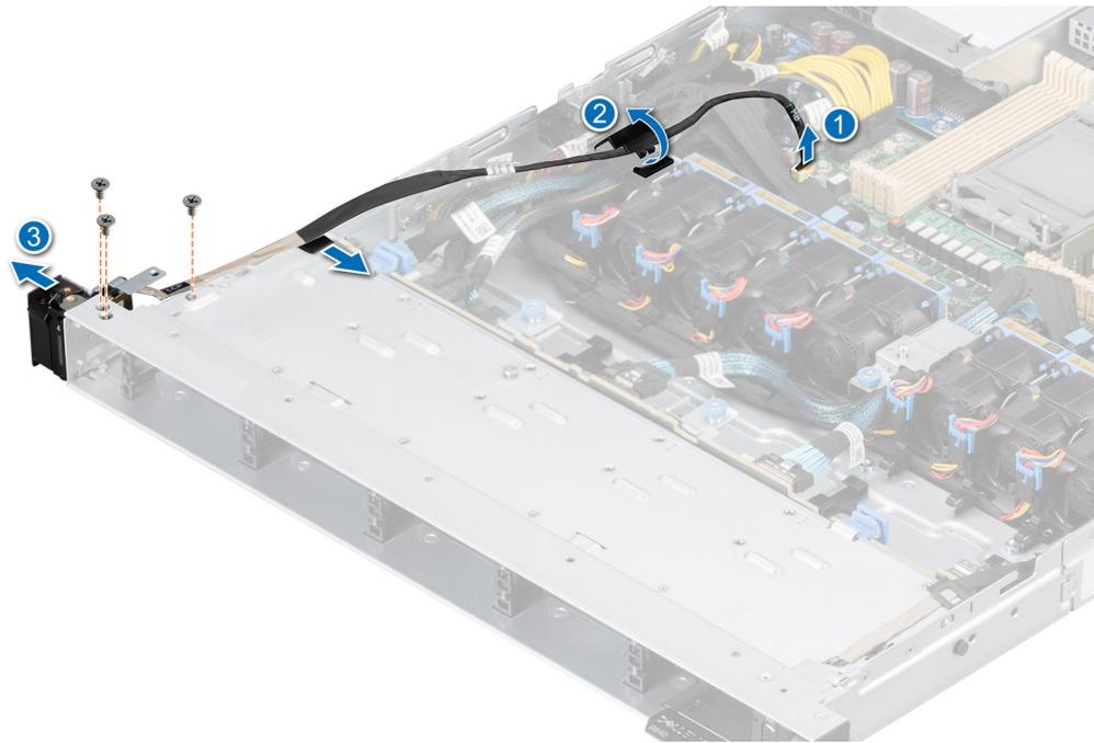
Figure 128. Removing the left control panel
