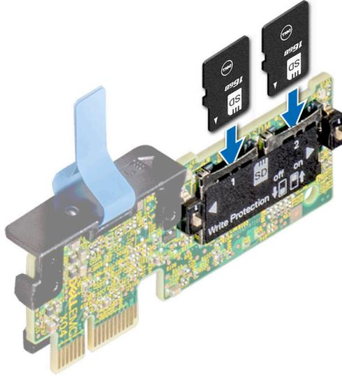
**Figure 100. Installing the MicroSD card**
