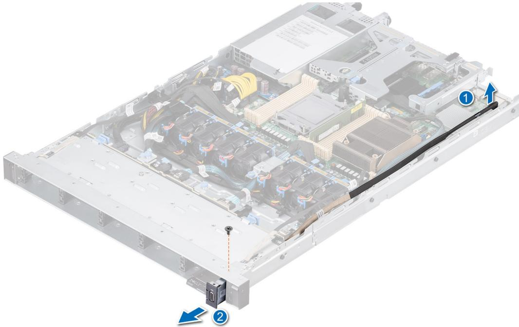
Figure 117. Removing the VGA module
