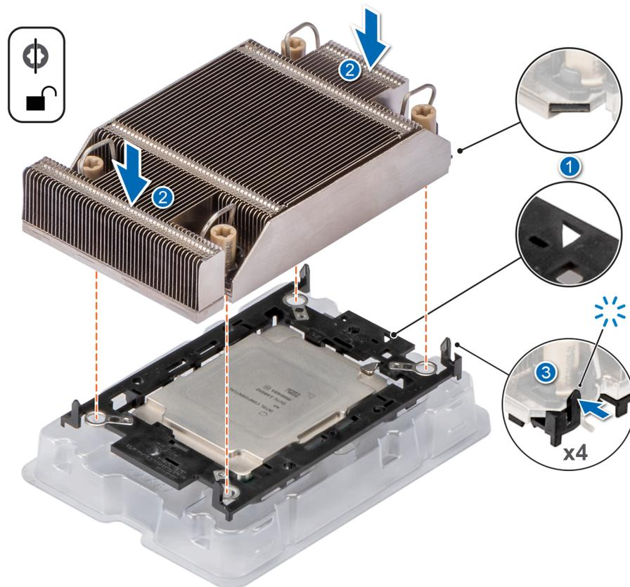
**Figure 61. Installing the heat sink onto the processor**
