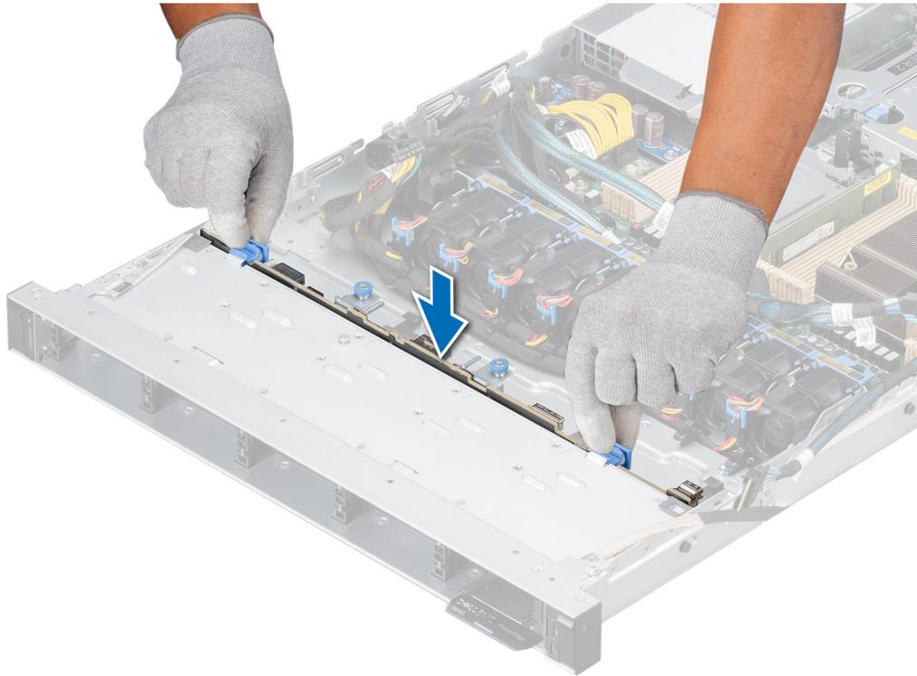
**Figure 36. Installing the drive backplane**
