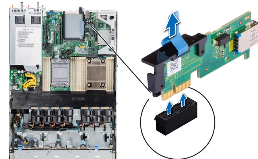
Figure 115. Removing the internal USB card
