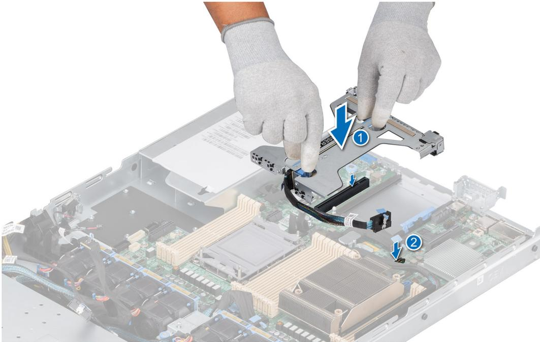
**Figure 75. Installing the Riser 2b with SNAP! module**
