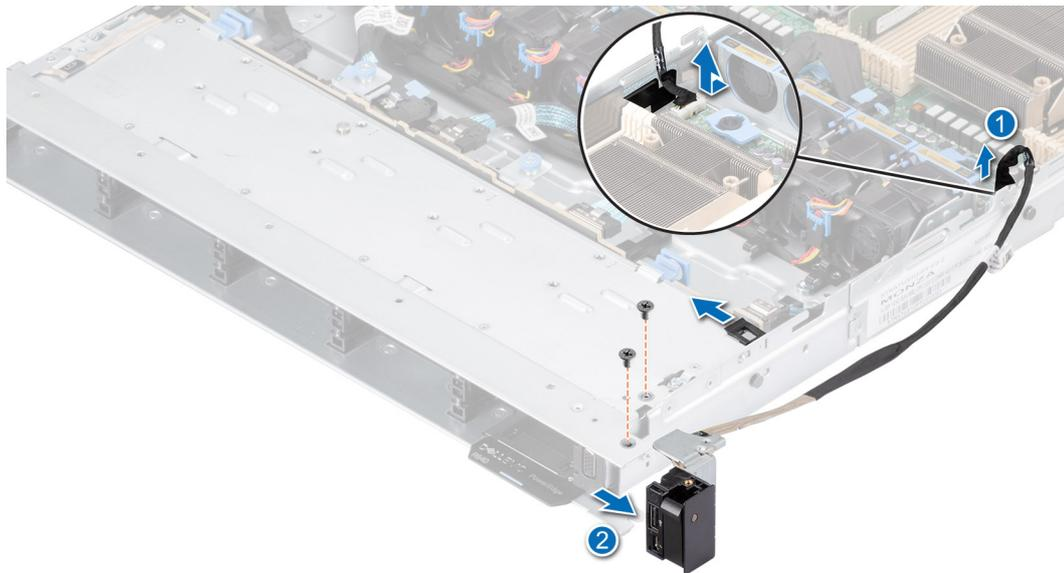
**Figure 130. Removing the right control panel**
