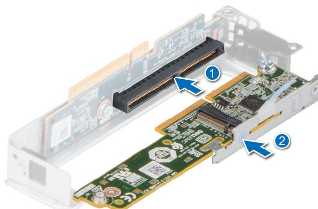
**Figure 104. Installing the M2 BOSS card into the M.2 BOSS riser**
