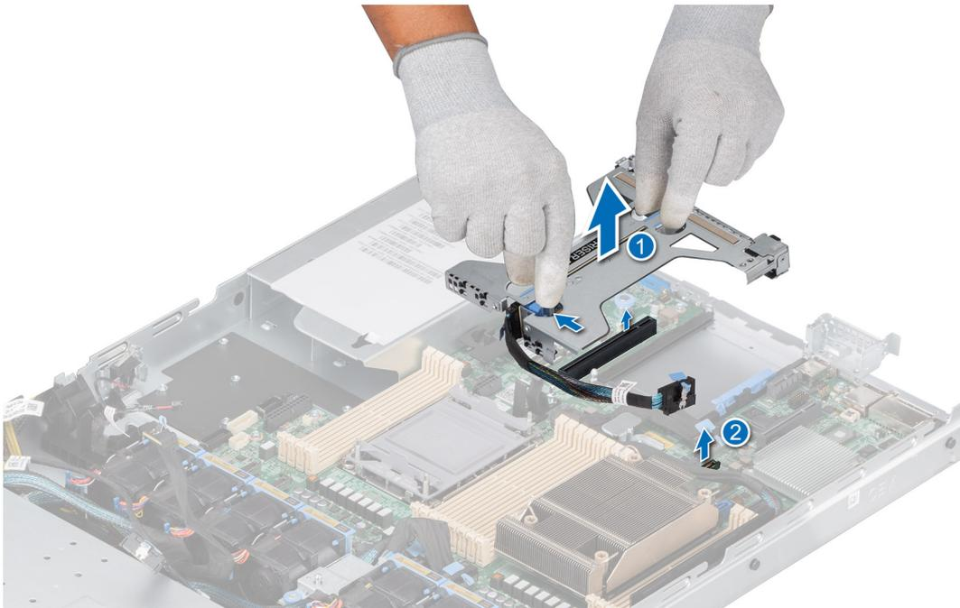
**Figure 71. Removing the Riser 2b with SNAPI module**
