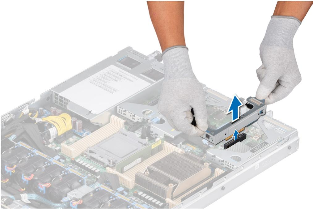
**Figure 101. Removing the M.2 BOSS riser**
