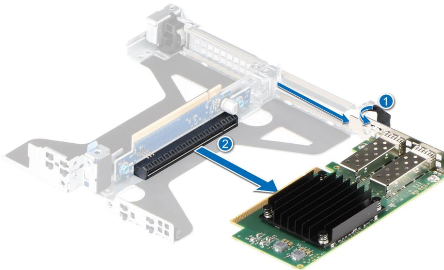
**Figure 80. Removing an expansion card from Riser 2c**
