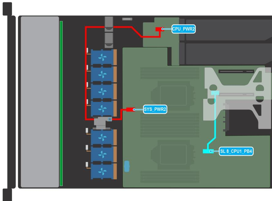
Figure 48. Cable routing - No drives with SNAPI riser
