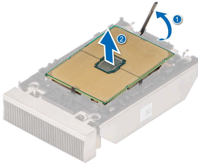
Figure 54. Lift the TIM break lever
