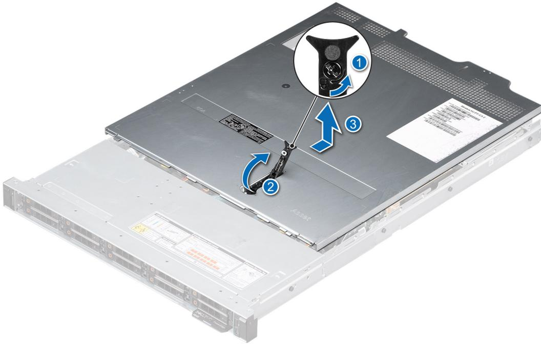
**Figure 14. Removing the system cover**
