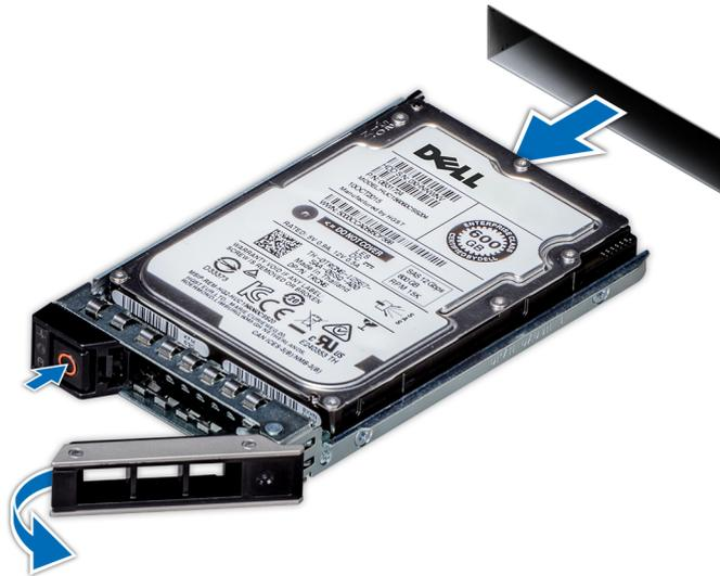
Figure 26. Removing a drive carrier
