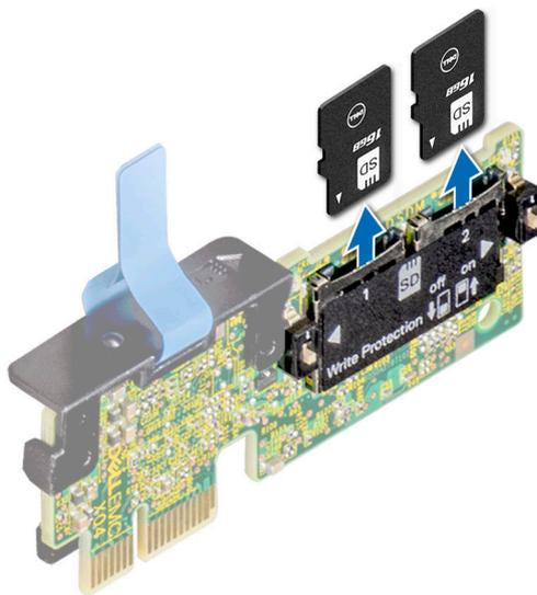
Figure 99. Removing the MicroSD card
