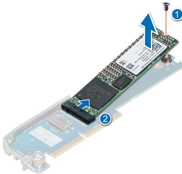
**Figure 105. Removing the M.2 SSD module**
