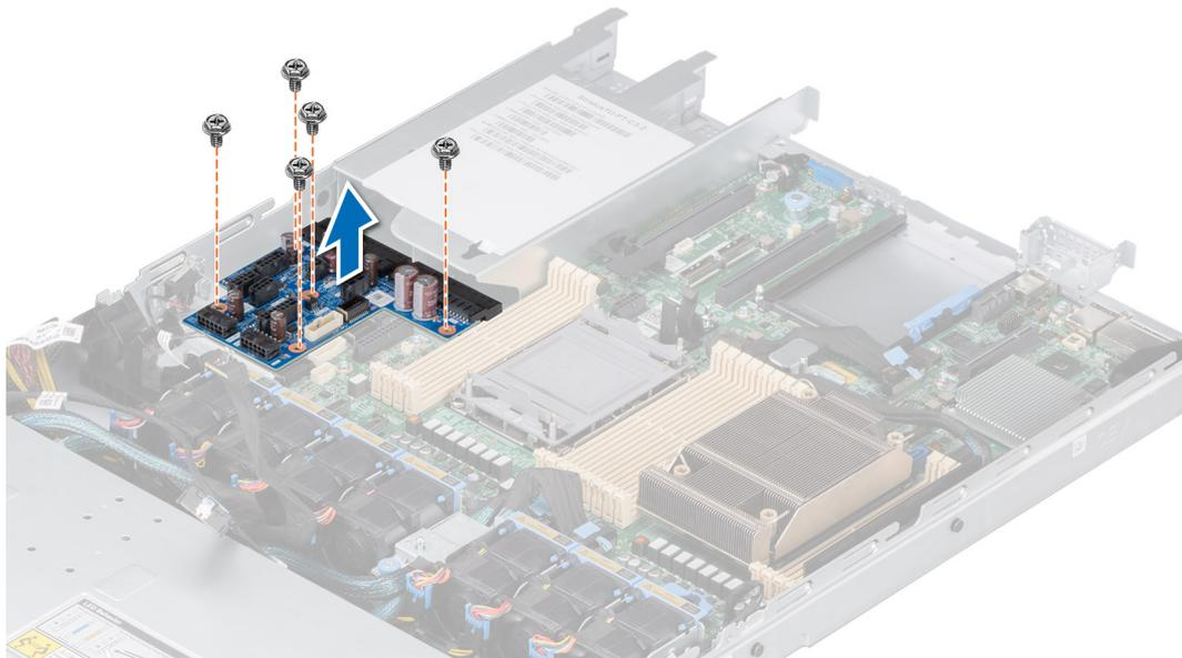
**Figure 123. Removing the power interposer board**
