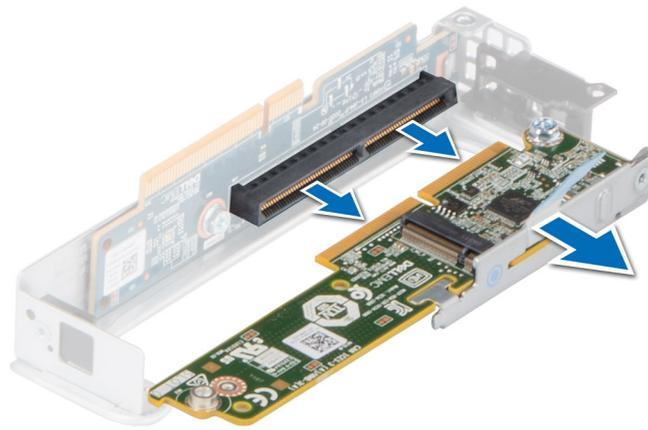
**Figure 103. Removing the M.2 BOSS card from the M.2 BOSS riser**
