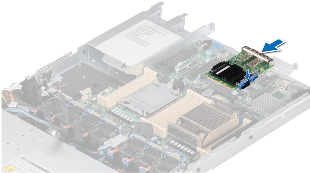
**Figure 110. Installing the OCP card**
