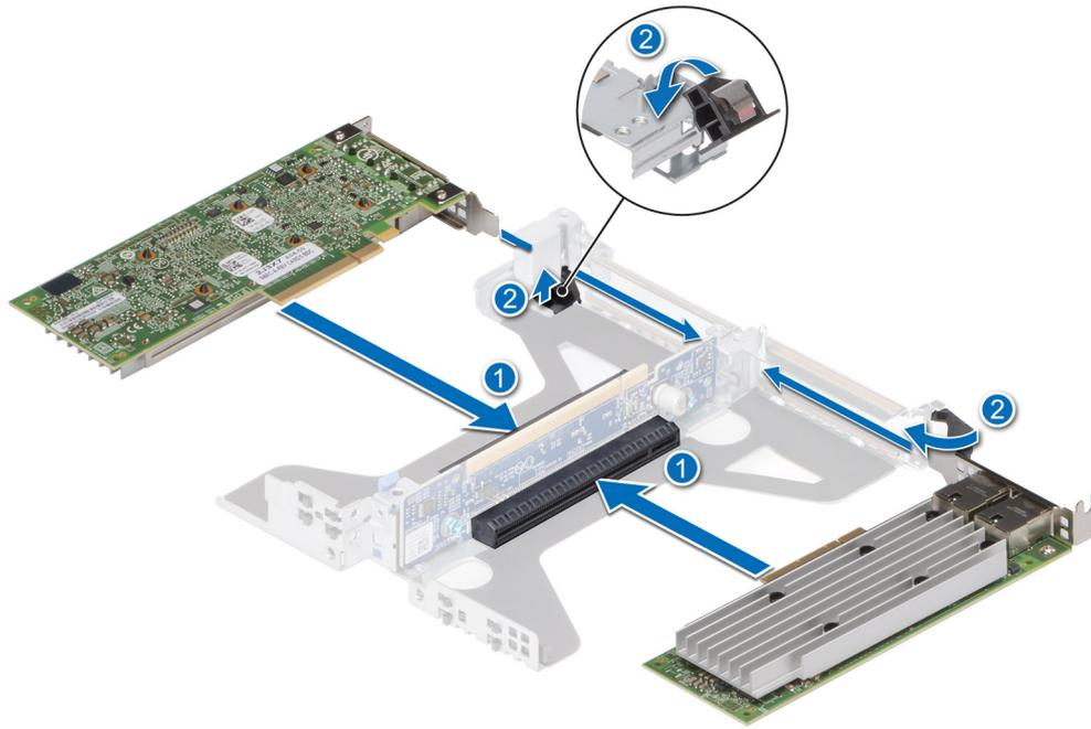
Figure 90. Installing an expansion card into a Riser 2a
