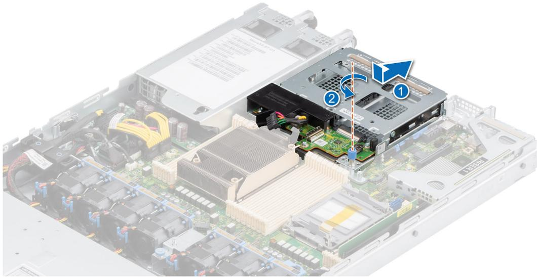
**Figure 94. Installing the 2.5-inch rear drive cage**
