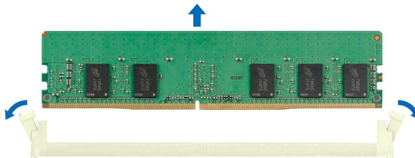
Figure 50. Removing a memory module
