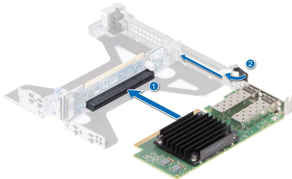
Figure 91. Installing an expansion card into a Riser 2b (SNAPI)
