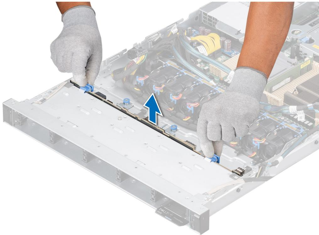
**Figure 35. Removing the backplane**
