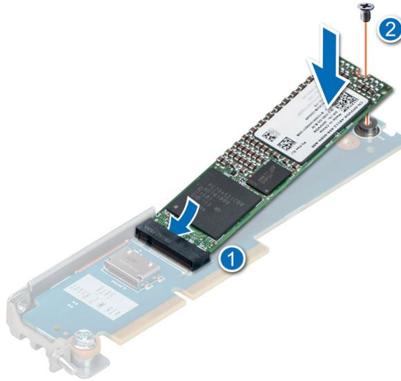
**Figure 106. Installing the M.2 SSD module**
