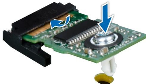
Figure 127. Installing the TPM
