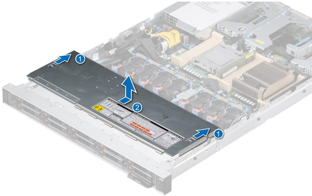
**Figure 16. Removing the drive backplane cover**
