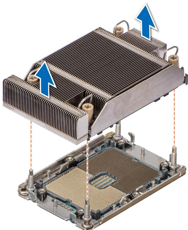
Figure 53. Removing a processor and heat sink module
