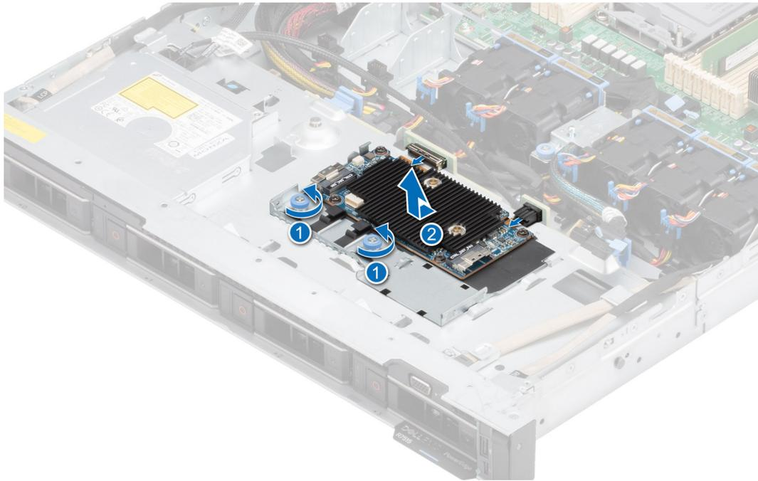
**Figure 111. Removing the front mounting front PERC module**
