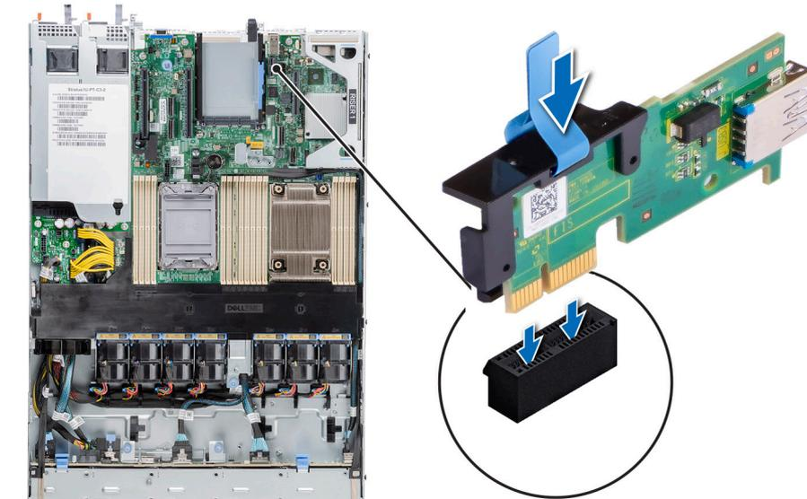
Figure 116. Installing the internal USB card
